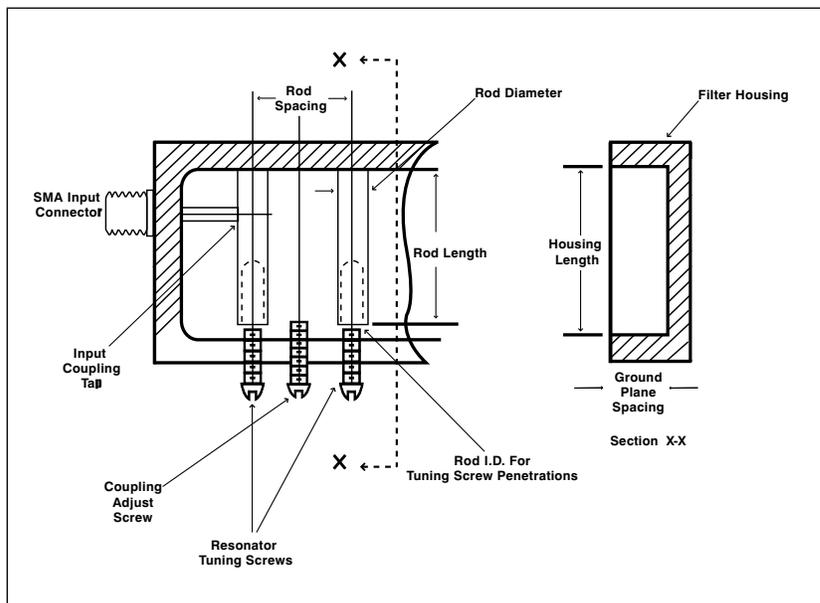
▲ **Figure 1. Mechanical details of the comblines band pass filter.**
