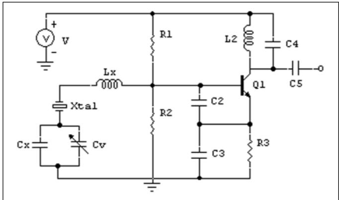
▲ Figure 2. Crystal oscillator circuit as a narrow-band modulator/transmitter.
