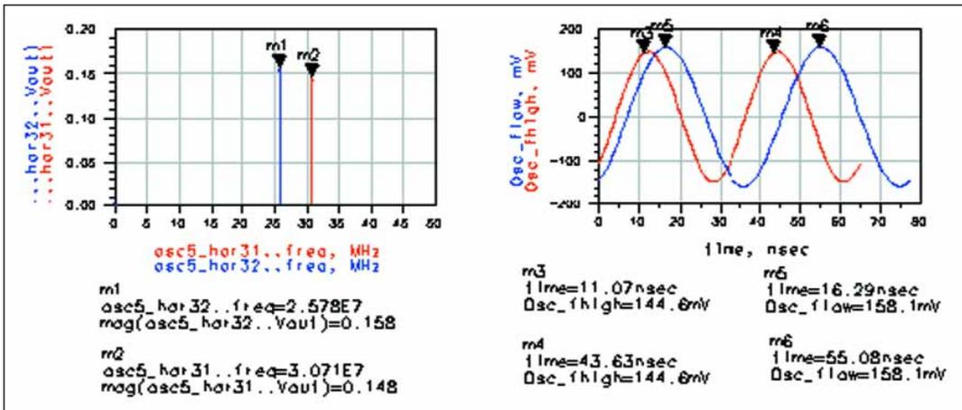
▲ Figure 5. Simulation results in the frequency domain (left) and time domain (right).
