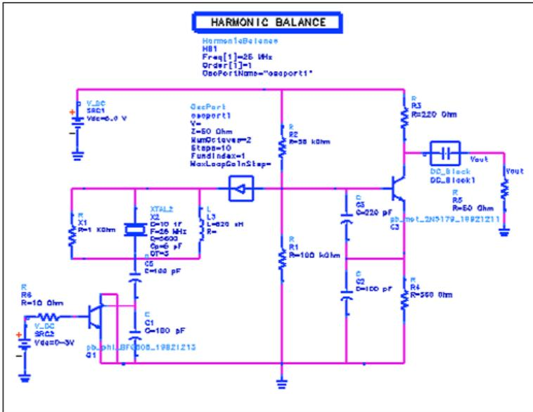
▲ **Figure 4.** Circuit simulation sets for HP ADS.
