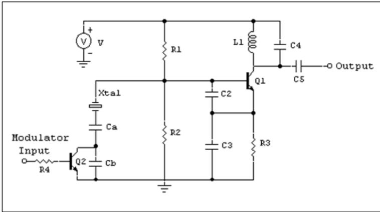
▲ **Figure 3.** A circuit with a new way to add value of capacitance that the circuit can accommodate.
