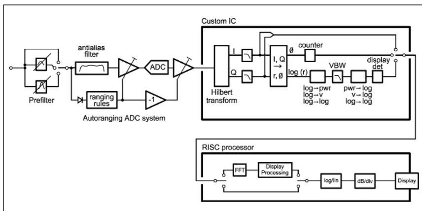
▲ **Figure 3.** Block diagram of the all-digital IF, with analog, custom ASIC and processor.
