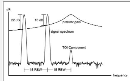
▲ **Figure A.** In swept TOI testing, when the analyzer is tuned to the TOI product, the interfering tones are attenuated 16 and 22 dB by the prefilter.
