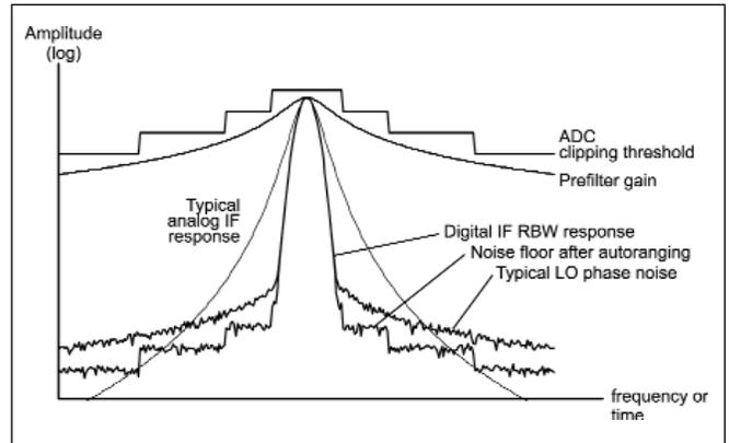
▲ **Figure 4. Autoranging keeps the ADC noise close to the carrier and lower than LO noise or RBW filter response.**
