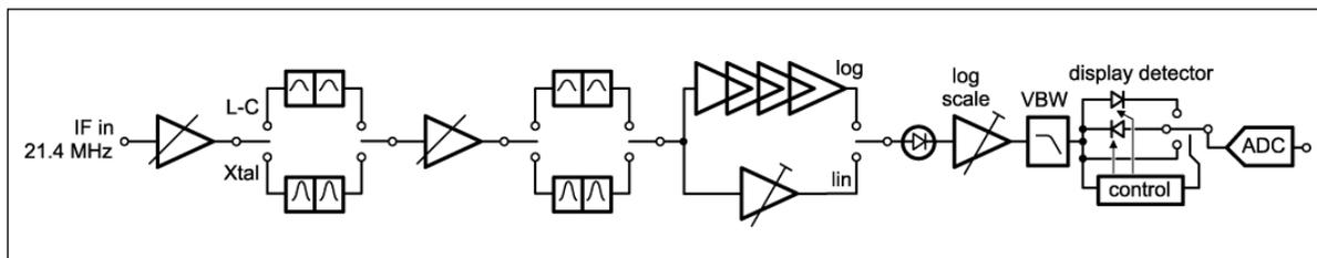
▲ **Figure 1.** An analog IF spectrum analyzer has step gains, L-C and crystal filters, log amps and detectors.
