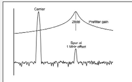
▲ **Figure C.** When the IF is tuned to a spurious component, it attenuates the carrier by so much that the ADC clipping-to-noise ratio does not affect the compression-to-noise.
