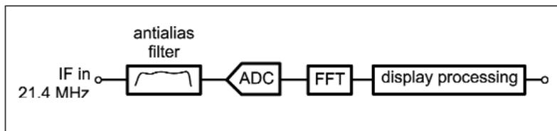
▲ **Figure 2.** An FFT-based IF digitizes the signal and computes the spectrum to be displayed.
