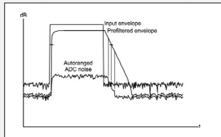
▲ **Figure B.** A pulsed-RF input signal is delayed by the prefilter, allowing the ADC ranging to follow. The effective ADC noise stays below visible levels (not to scale).
