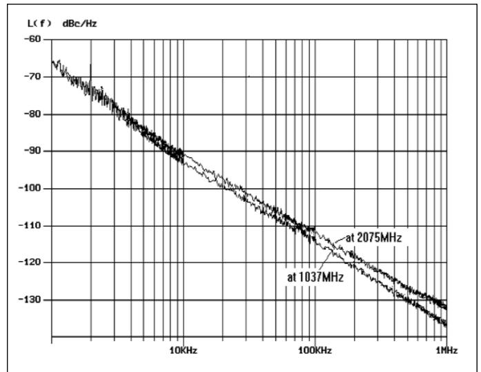
▲ Figure 15. RF VCO phase noise plot at  $V_{CTL} = 1.5$  V and  $V_{CC} = 3$  V.
