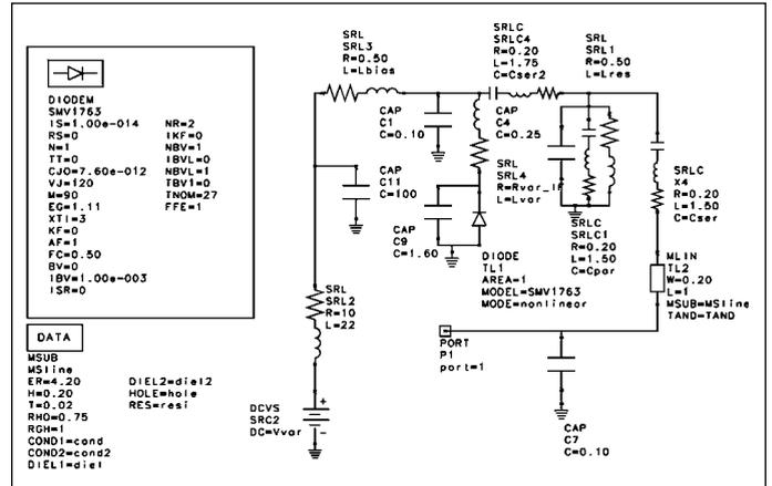
▲ Figure 4a. The RF VCO resonator model.
