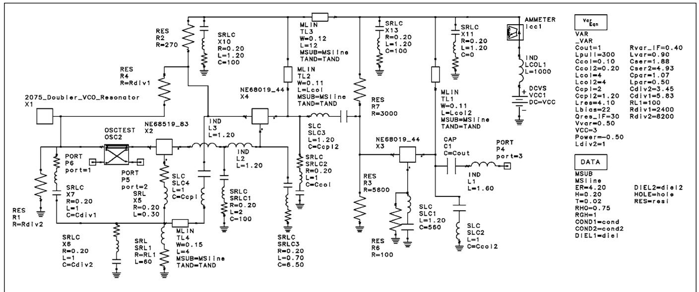
▲ Figure 4b. The RF VCO circuit model.
