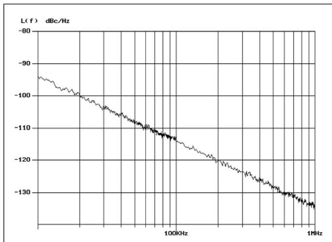
▲ Figure 18. IF VCO phase noise plot at  $V_{CTL} = 1.5$  V and  $V_{CC} = 3$  V.
