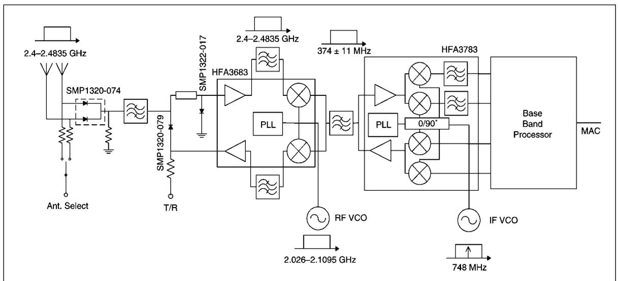
▲ Figure 1. Typical WLAN RF interface architecture based on the Intersil Prism™ chip set [2].
