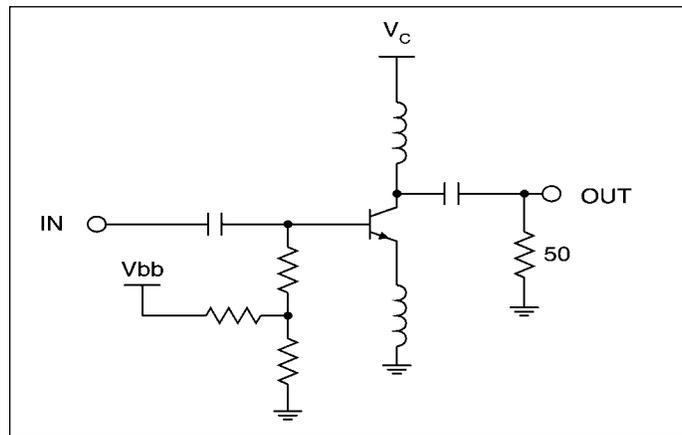
▲ **Figure 2. Single-stage amplifier circuit used for analysis of self-biasing.**
