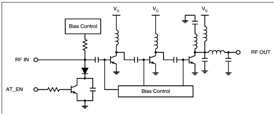
▲ Figure 5. Circuit of the improved amplifier with a PIN diode attenuator.
