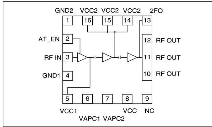
▲ Figure 7. Pinout diagram of the RF2140/2174.
