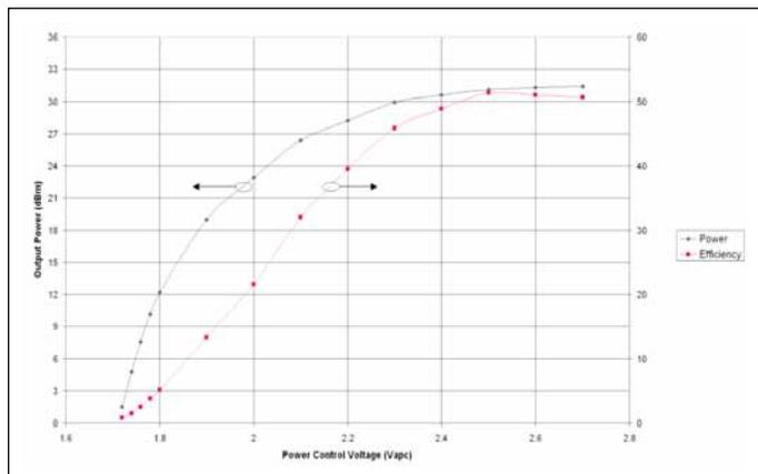
▲ Figure 9. Measured output power and power-added efficiency (PAE) for  $V_{CC} = 2.7$  V.
