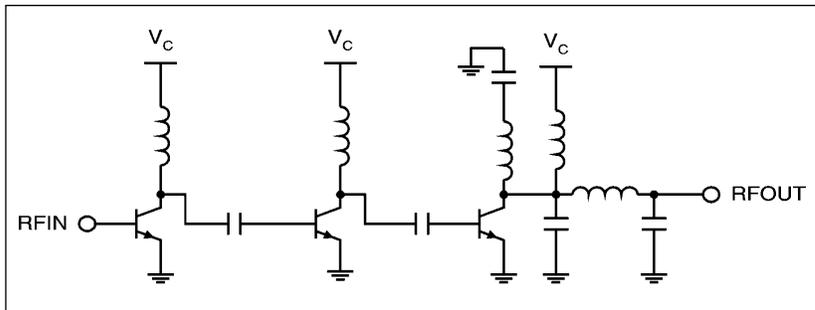
▲ Figure 1. Simplified circuit diagram of a three-stage power amplifier.
