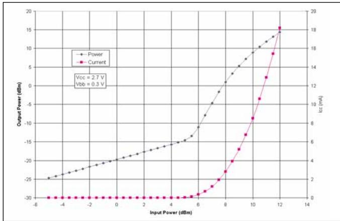
▲ Figure 3. Power output and collector current vs. power input at  $V_{CC} = 2.7$  volts.
