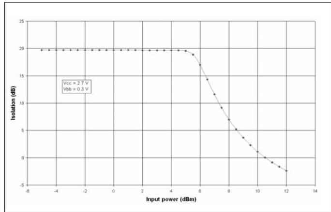
▲ Figure 4. Isolation as a function of input power, showing the rapid degradation above 6 dBm input.
