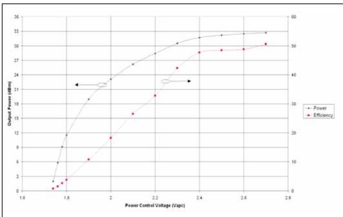
▲ Figure 8. Measured output power and power-added efficiency (PAE) for  $V_{CC} = 3.2$  V.
