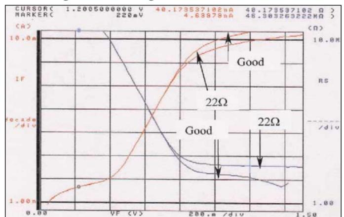
▲ Figure 15. The resistance plot shows an offset equivalent to 39 ohms (diode internal resistance plus 22 ohms loss.)
