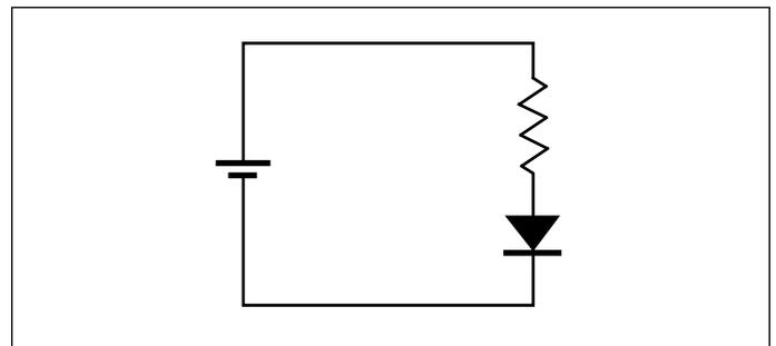
▲ Figure 13. High series resistance equivalent circuit.
