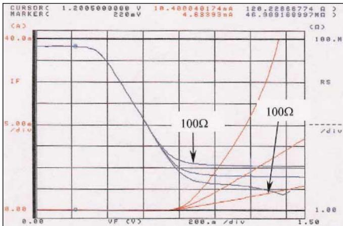
▲ Figure 16. I/V plots comparing a good diode with an additional loss due to 100 ohms series resistance.
