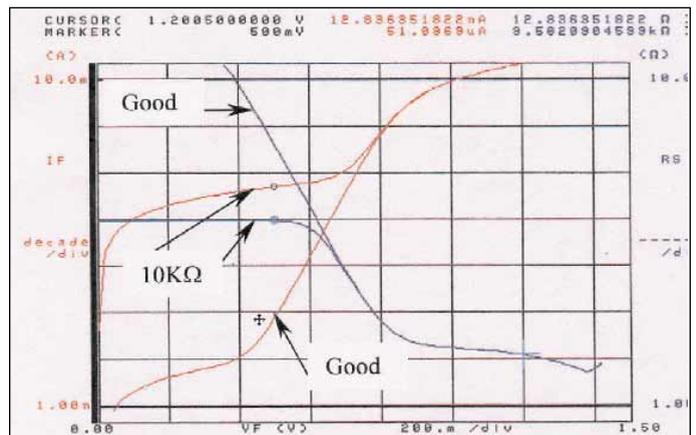
▲ Figure 6. Resistance curve of a leaky diode with  $10\text{ kohm}$  parallel resistance.
