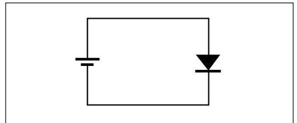
▲ **Figure 1. DC equivalent circuit for a diode.**
