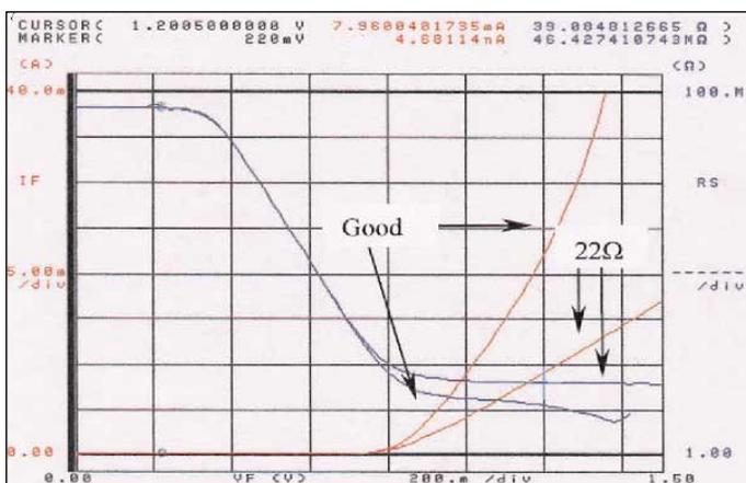
▲ Figure 14. I/V curves with a good diode and one with an additional 22 ohms series resistance.
