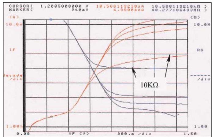
▲ Figure 19. Resistance plot shows a large deviation from behavior of a good diode.
