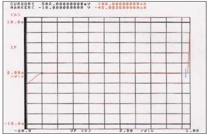
▲ Figure 3. I/V plot scaled to show breakdown voltage and forward voltage drop.
