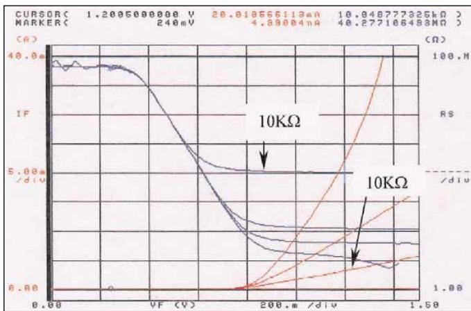
▲ Figure 18. I/V curves with the bad diode having 10 kohm series resistance.
