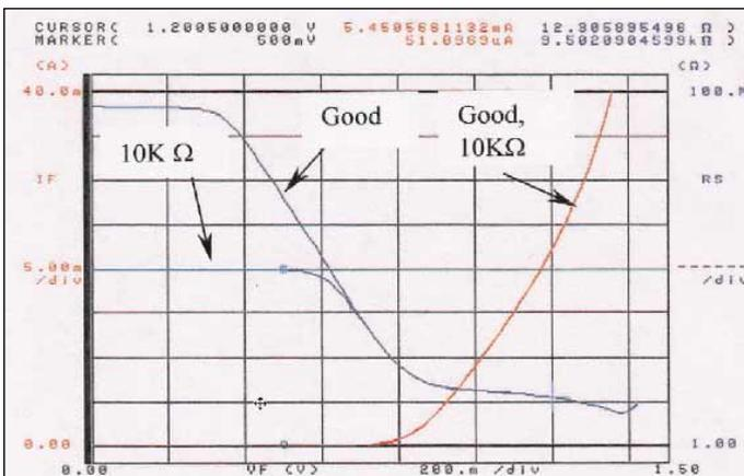
▲ Figure 5. Leaky diode I/V curve with  $10\text{ kohm}$  parallel resistance.
