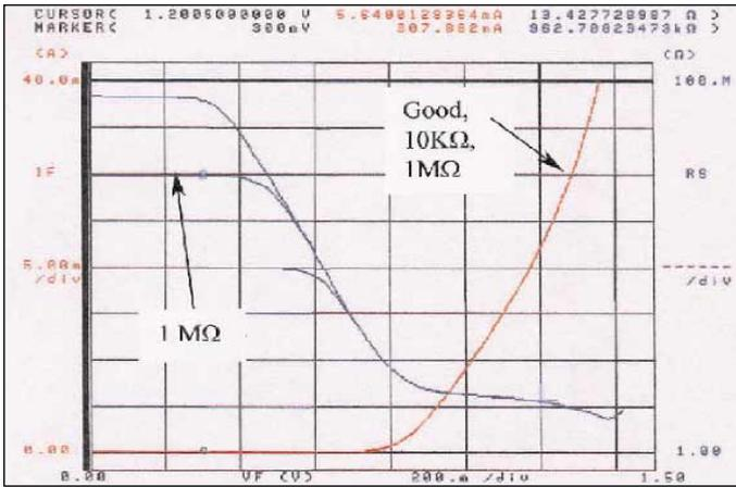
▲ Figure 7. I/V curve with leakage represented by a 1 Mohm resistor.
