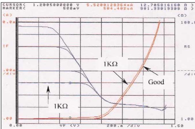
▲ Figure 9. I/V curves with leakage represented by a 1 kohm resistor.
