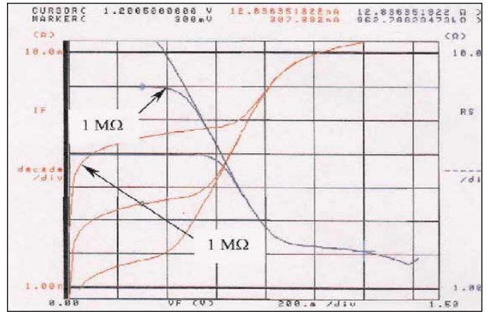
▲ Figure 8. A log scale graph clearly shows the leakage due to 1 Mohm parallel resistance.
