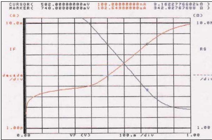
▲ Figure 2. I/V curve (red) and resistance curve (blue) of a good diode.
