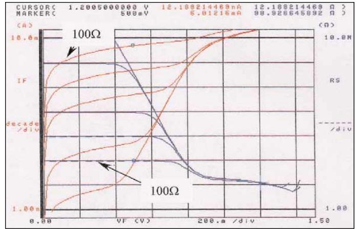
▲ Figure 12. On a log scale, the leakage due to 100 ohm parallel resistance is clearly shown.
