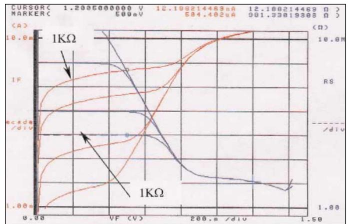
▲ Figure 10. A log scale graph shows the greater leakage with the lower parallel resistance.
