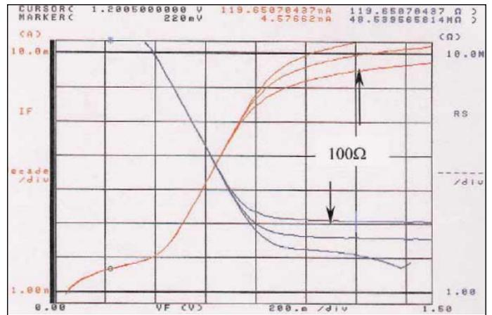
▲ Figure 17. Resistance plot shows the additional 100 ohm series resistance
