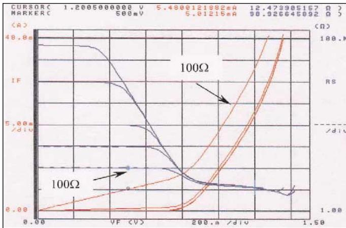
▲ Figure 11. 100 ohm parallel resistance show clear variation on the I/V curve.
