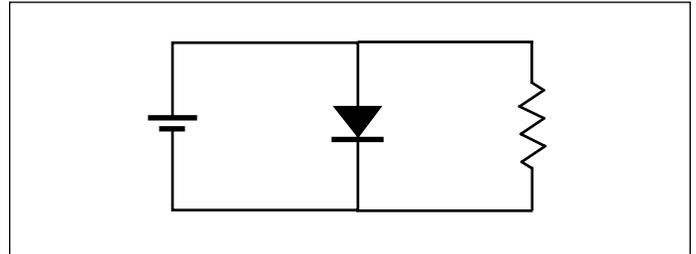
▲ Figure 4. Equivalent circuit of a leaky diode with a parallel resistor.
