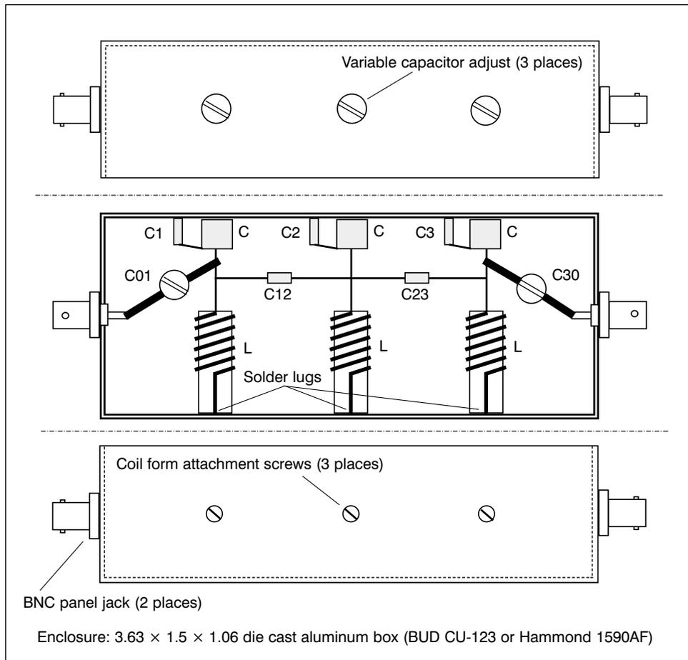
▲ **Figure 3. Bandpass filter mechanical construction details.**
