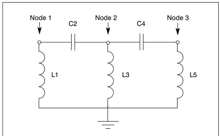
▲ **Figure 1. Highpass filter schematic.**
