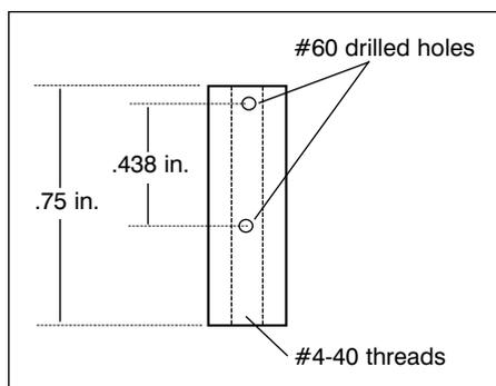
▲ **Figure 4. Preparation detail of the nylon spacer used as a coil form (three required).**
