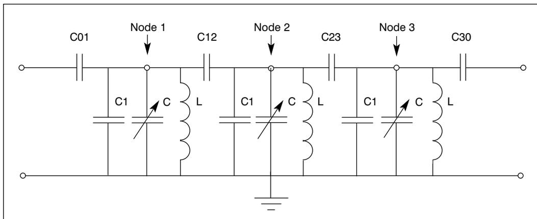
▲ Figure 2. Schematic of the 70 MHz bandpass filter example.
