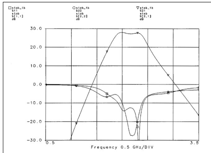
▲ Figure 5. Measured small signal S parameters for the S-band two-stage amplifier, showing the typical bandpass gain obtained with this method.
