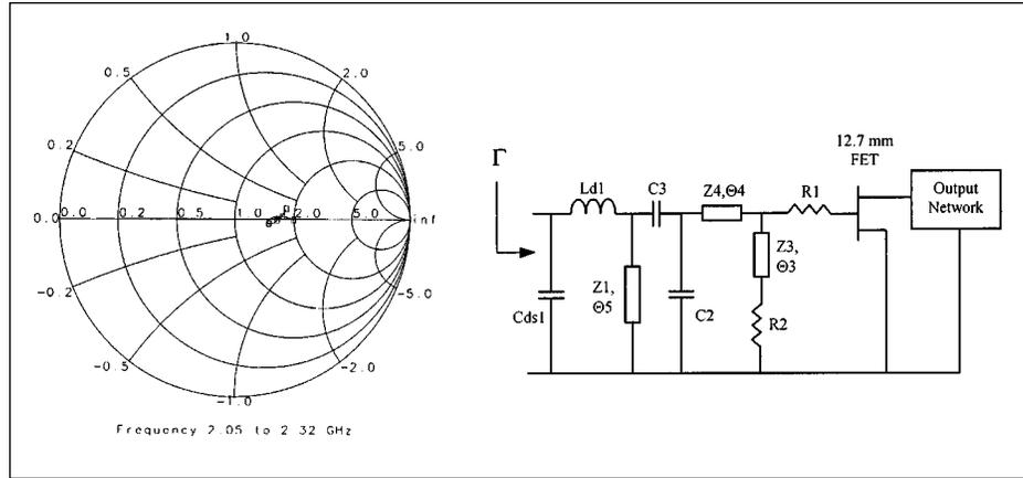
▲ Figure 2. Desired impedance locus for wide band interstage matching with de-embedded first stage parasitic elements  $Cds_1$  and  $Ld_1$ .
