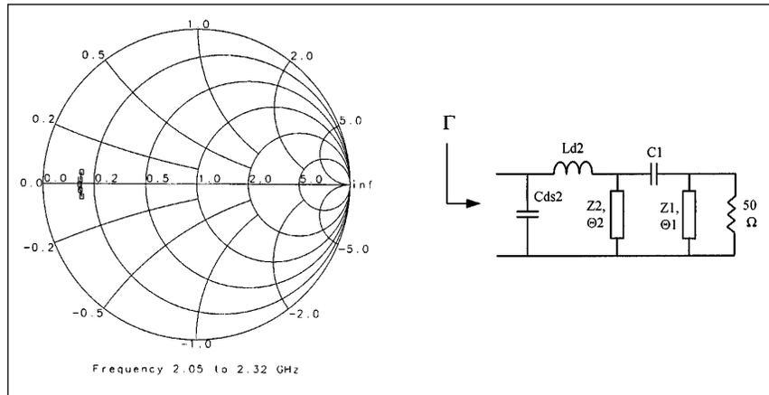
▲ **Figure 1. Desired impedance locus for output matching of the second stage with de-embedded parasitic elements  $Cds_2$  and  $Ld_2$ .**
