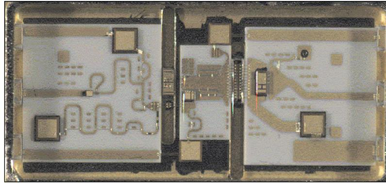
▲ Figure 4. Photograph of the hybrid MIC S-band amplifier with 26 dB small signal gain, 60 percent power-added efficiency and 0.5 dB gain flatness over a 10 percent bandwidth.
