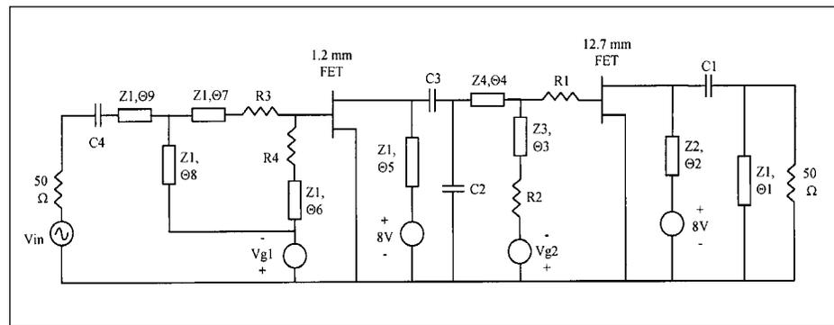
▲ Figure 3. Complete amplifier topology showing the high pass output matching network, combination interstage network, stability network and bandpass input matching network.
