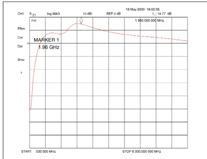
▲ Forward gain, wide span (30 kHz to 6 GHz).
