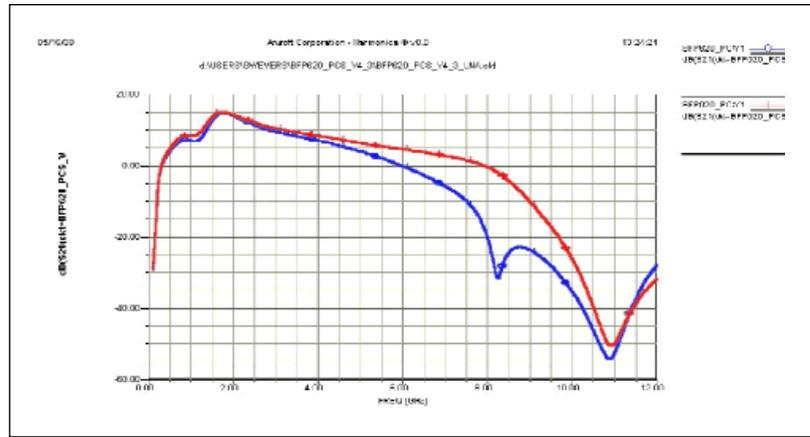
▲ **Figure 7. Simulated plot of LNA gain showing effect of capacitor C7 on high frequency gain of LNA.**
