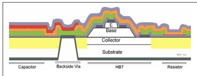
▲ Figure 3. Cross section of TRW/RFMD GaAs HBT.
