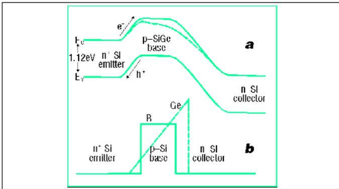
▲ Figure 1. Band gap energy profile. (Source: IBM)
