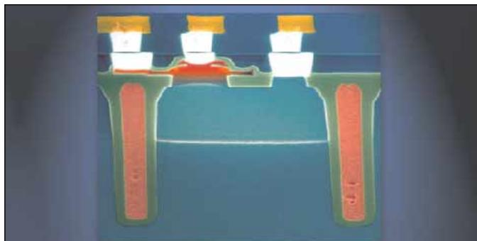
▲ SiGe Cross section from IBM 5HP process. (Source: IBM)
