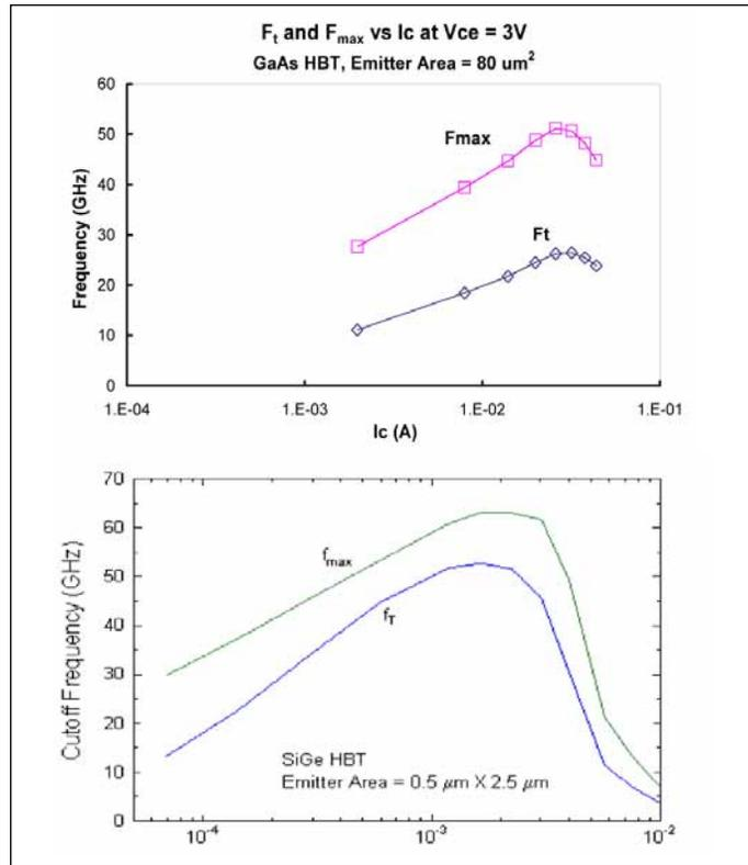
▲ Figure 5. GaAs/AlGaAs HBT (top) and SiGe (bottom) cutoff frequency vs. collector current. (Source: IBM)
