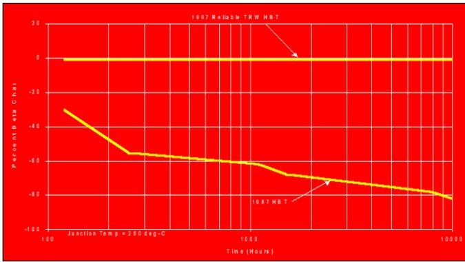
▲ Figure 6. DC Beta degradation vs. time.
