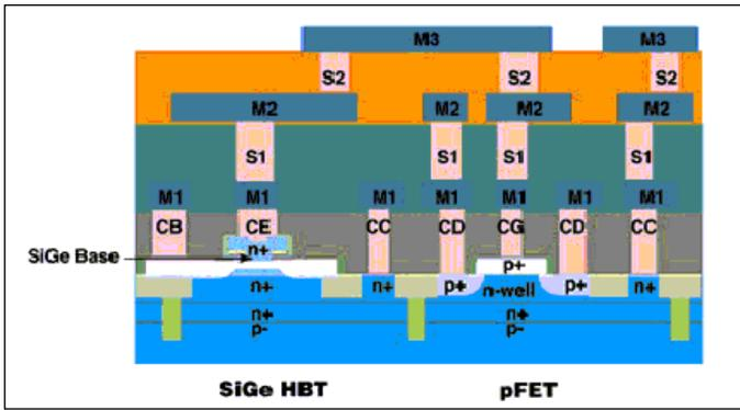
▲ Cross section of the SiGe HBT transistor. (Source: IBM)
