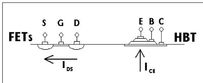
▲ **Figure 8. HBT structure provides a more efficient usage of chip area for current handling.**
