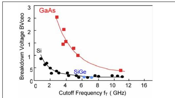
▲ Figure 4. Breakdown voltage vs.  $f_T$ . (Source: TRW)
