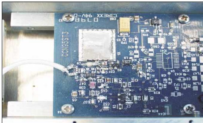
▲ **Figure 9.** Photograph of the oscillator as constructed.
