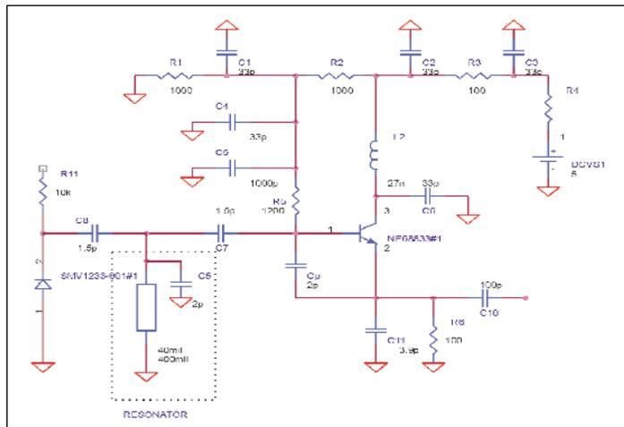
▲ Figure 1. The resonating structure used in the oscillator keeps cost down while achieving low phase noise performance essential to wireless design.
