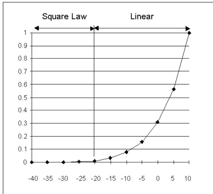
▲ **Figure 3. Diode response showing detected voltage vs. input power (dBm).**
