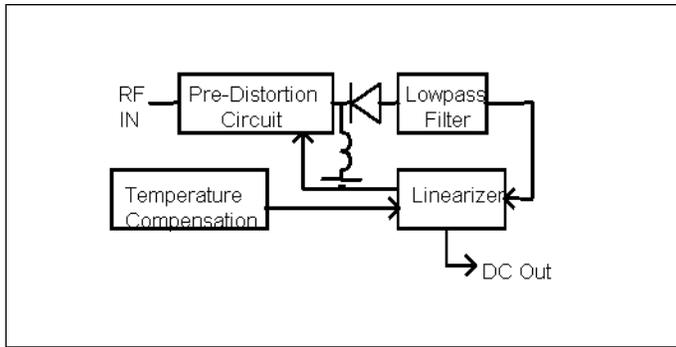
▲ Figure 4. PDM block diagram.
