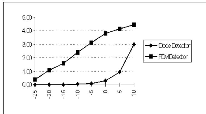
▲ Figure 8. PDM vs. diode response showing detected voltage vs. input power (dBm).
