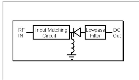
▲ **Figure 1. Diagram of a simple diode detector.**
