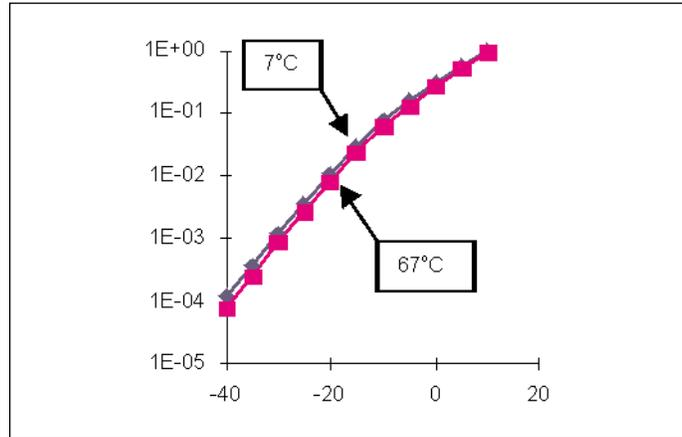
▲ Figure 5. Diode temperature performance showing detected voltage vs. input power (dBm).
