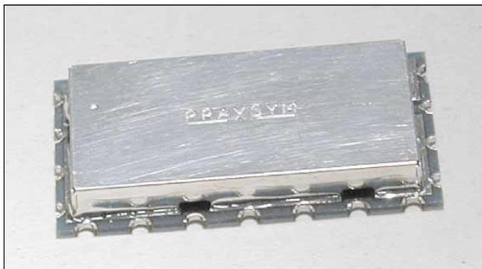
▲ Figure 7. PDM shielding.
