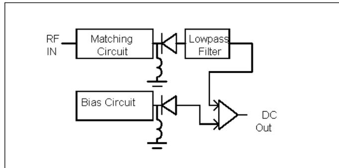
▲ Figure 6. Dual diode compensation.
