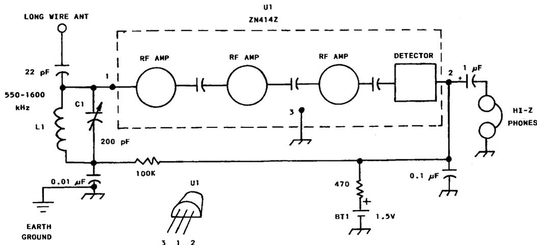
**FIGURE 1:** Circuit for a simple TRF radio using the Plessey ZN414Z 10-transistor IC. L1 consists of 131 close-wound turns of no. 20 enamel wire on a 5-1/2 inch length of 2-3/8 inch OD PVC tubing. L1 has 420 microhenries of inductance for tuning from 550 to 1600 kHz with a 200-pF variable capacitor (see text for toroidal coil data). The audio amplifier in Figure 2 can be added for greater headphone volume, and to permit using 8-ohm phones. Omit RFC1 if this is done.
