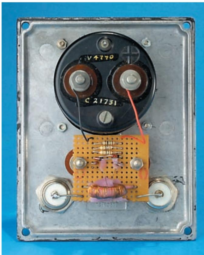
● Fig. 4: A close up of the simple layout of the current sensing transformer, rectifiers, and loading resistors.
