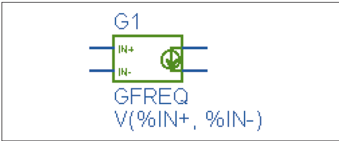
▲ Figure 3. SPICE A/D symbolic representation of a frequency-dependent voltage controlled current source.
