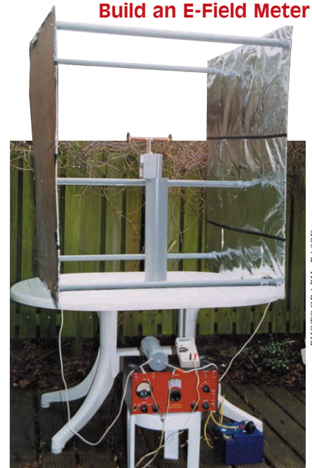
Set-up for calibration. Below can be seen the QRP transmitter with balun and digital voltmeter on top.
