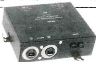
New hi-volt power supplies made by Wabash Co. Their original use was probably to electrify the coronas in a photo-copy machine. The high voltage nature of this device should "spark" your imagination - small lasers or bug zappers, etc. Input 115 V, 60 Hz. Output 13.5 KV 0.5 ma. Shpg. Wt. 6 Lbs SPL-470-33A \$12.00
