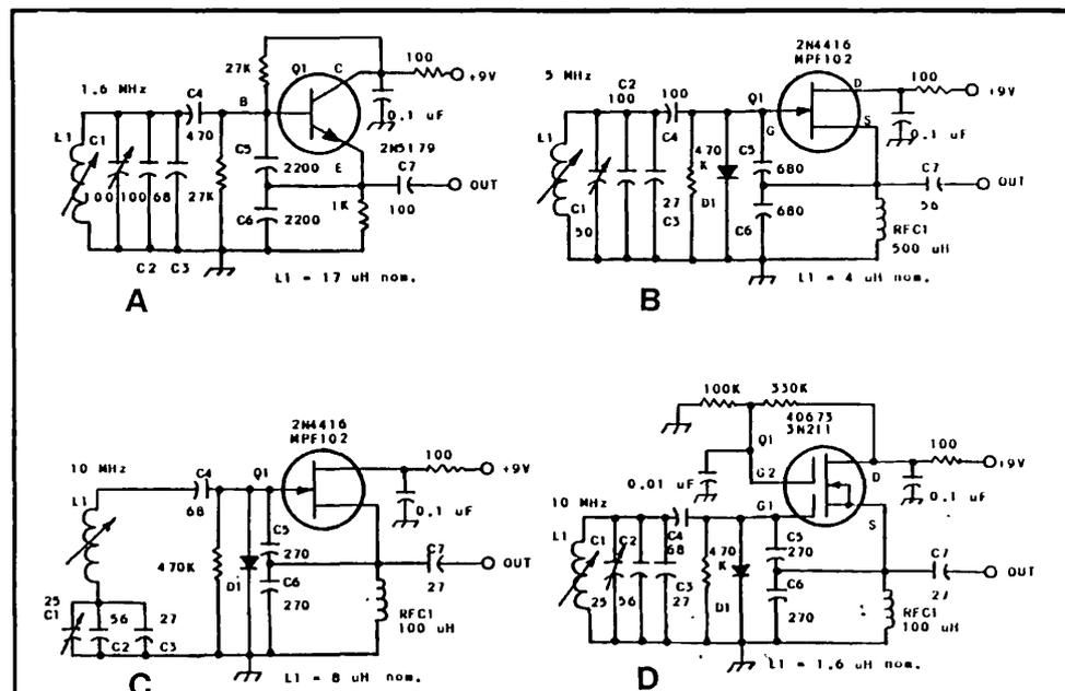
**Fig 1** - Schematic diagrams of four versions of the Colpitts oscillator. Circuits A, B and D are parallel tuned. Circuit C is series tuned. Compare C to D to learn how the L1 inductance changes when using a series-tuned circuit. All other component values remain the same, as does the operating frequency (see text).
