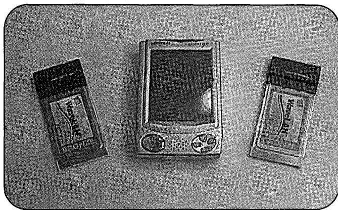
HSMM HT: In the center is the well-recognized PDA (Personal Data Assistant), or hand-held PC. This one, however, is equipped to work on 2.4 GHz using IEEE 802.11 PCMCIA cards. One of these cards (essentially, the cards are the transceiver RF section in a module) and some software turns this PDA into a potential amateur radio HSMM HT.
