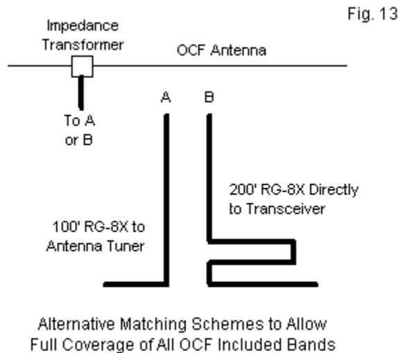
**Fig. 13** shows the options that we have. We may run the 100' of cable to an antenna tuner to obtain a quite precise 50-Ω impedance at all operating frequencies. Alternatively, we may use 200' of RG-8X directly to the transceiver and still obtain full band coverage of all included operating segments. The SWR will not be 1:1 at every frequency, but it will be less than 2:1 across every included band.
