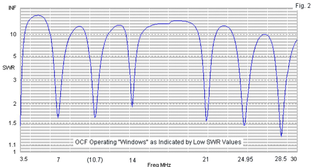
I have added markers on the frequency line to indicate potential operating windows. Six of them fall within amateur bands. Unfortunately, the window at 10.7 MHz is too high to allow use of the antenna on 30 meters. We should also note that each of the operating windows is fairly narrow. Some of them may not be wide enough or reach SWR values low enough to let us use the entire band as we measure such values at the impedance transformer.
