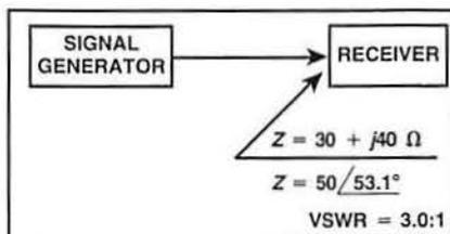
Figure 1. The receiver input presents a complex impedance of  $(30 + j40)$  ohms to the signal generator. This causes an SWR of 3:1. The complex impedance is also shown in polar form as  $50\Omega$  at an angle of  $53.1^\circ$ .
