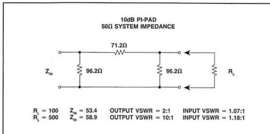
Figure 4. This shows how a 10dB pad would reduce the VSWR for a load of  $100\Omega$  or  $500\Omega$ . The  $100\Omega$  load would normally cause a VSWR of 2:1, but the 10dB pad reduces the VSWR to 1.07:1. The  $500\Omega$  load would cause a VSWR of 10:1, but the 10dB pad reduces it to 1.18:1 at the input.
