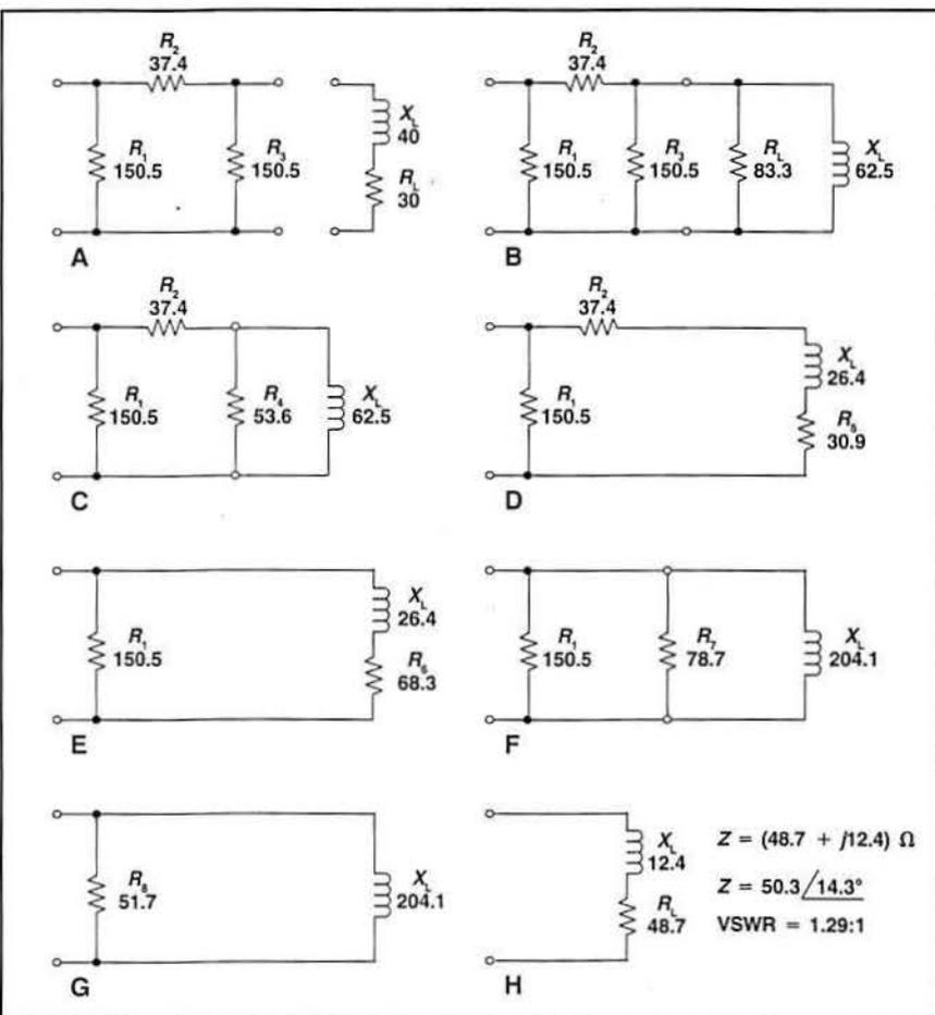
Figure 3. This illustrates through evolution how a 6dB pad transforms the output impedance to the impedance that is "seen" at the pad input. The output impedance,  $(30 + j40)$  ohms, would cause a VSWR of 3:1. However, looking at the input to the pad, the generator or source would see an impedance of  $48.7 + j12.4$  ohms for a VSWR of 1.29:1.
