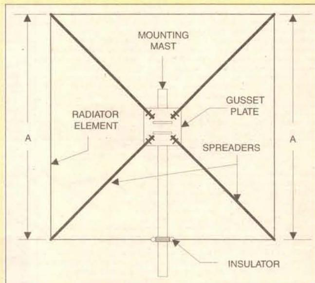
Figure 1 - Rotatable quad loop antenna.
