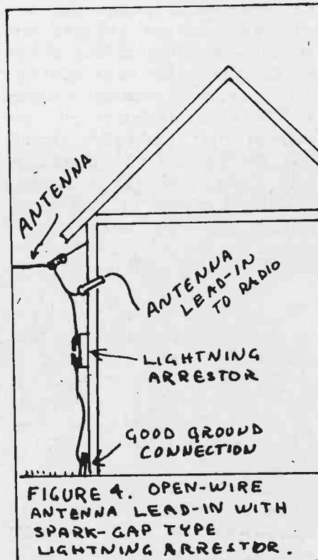
**FIGURE 4. OPEN-WIRE ANTENNA LEAD-IN WITH SPARK-GAP TYPE LIGHTNING ARRESTOR.**
