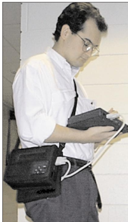
▲ Figure 5. A pen-based computer and test receiver are used to input actual signal measurement data into SitePlanner.
