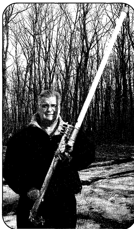
Gary Blacksmith, WA3CPO, holding the 23-cm omni antenna. It is designed to be well protected from intruding insects.
