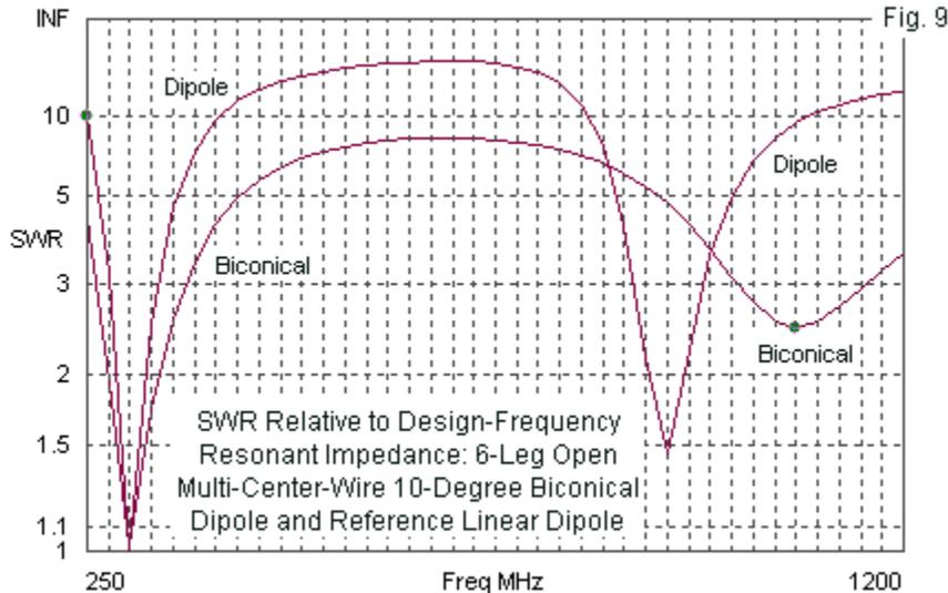
The second low-impedance resonance for the linear dipole occurs at about 925 MHz (using 25-MHz increments for the sweep). The comparable resonant frequency for the biconical dipole is about 1075 MHz. The increment between the -10-dB limit frequency and the second resonance frequency increases as we add legs to the biconical model.
