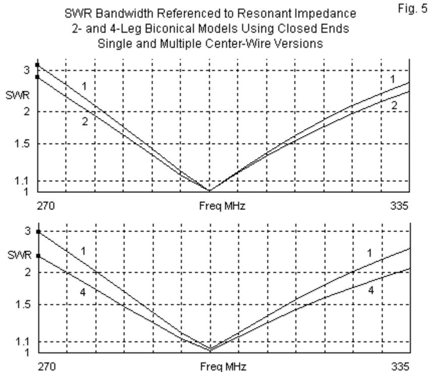
I noted in passing that we need not model past 4 or 6 legs to obtain a reasonable approximation of a full conical structure. To confirm this suggestion--and to note its limits--let's draw together the data for multi-wire center models of 4-leg and 6-leg  $10^\circ$  biconical antennas with both open and closed ends. For each number of legs, we may place side-by-side the data for open and closed end models. **Table 5** supplies the numbers.
