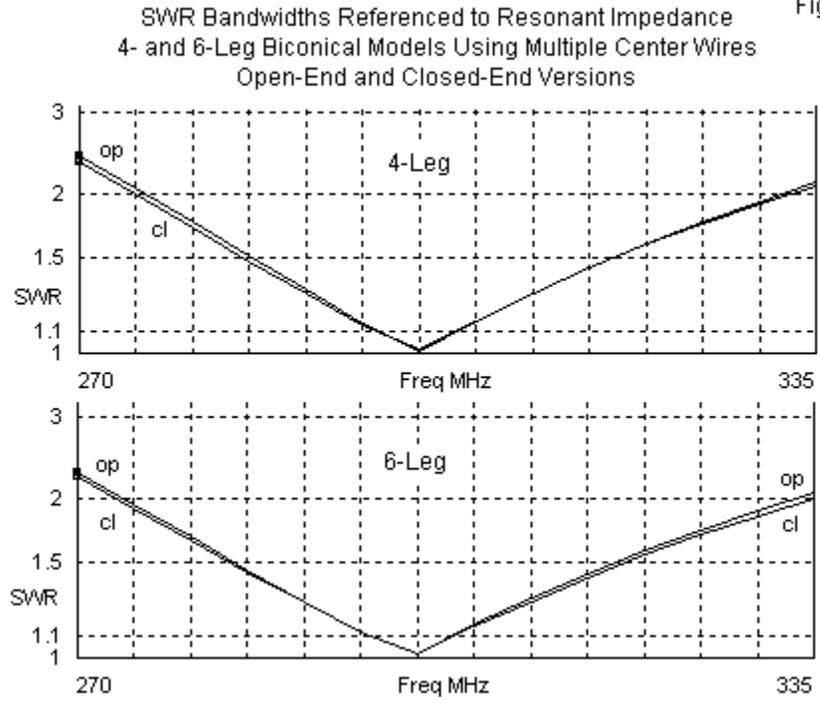
Equally apparent is the fact that a 6-leg model shows only a tiny increment of improved SWR performance over its 4-leg counterpart along with only a 1-Ω difference in the feedpoint
