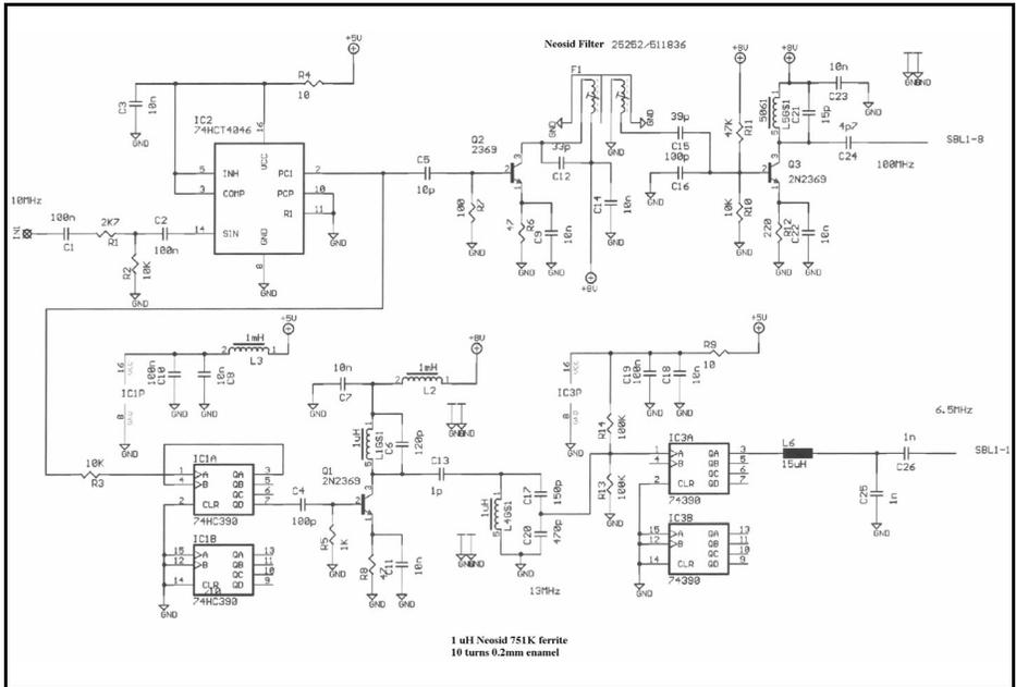
**Fig 4a: Circuit diagram of local oscillator.**
