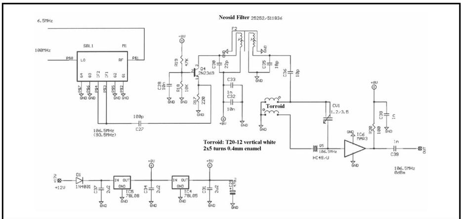
**Fig 4b: Circuit diagram of local oscillator.**
