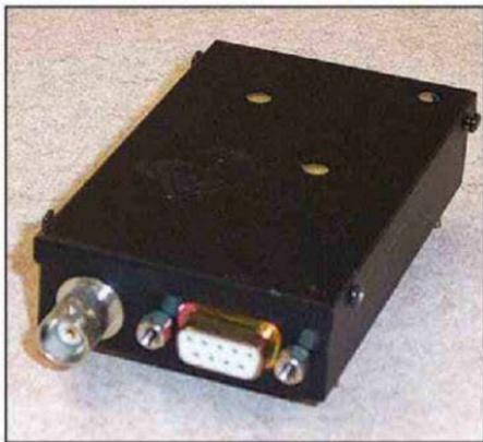
Fig. 1. A TEKK KS-900 (T-Net Micro) data radio. This is a 2-watt crystal-controlled data radio that runs 9600 Baud out of the box, and can be tweaked to push 19,200 Baud. For several years, this was the best one could hope for when running packet backbone links on 70 centimeters. The DE-9F connector is for power and data.
