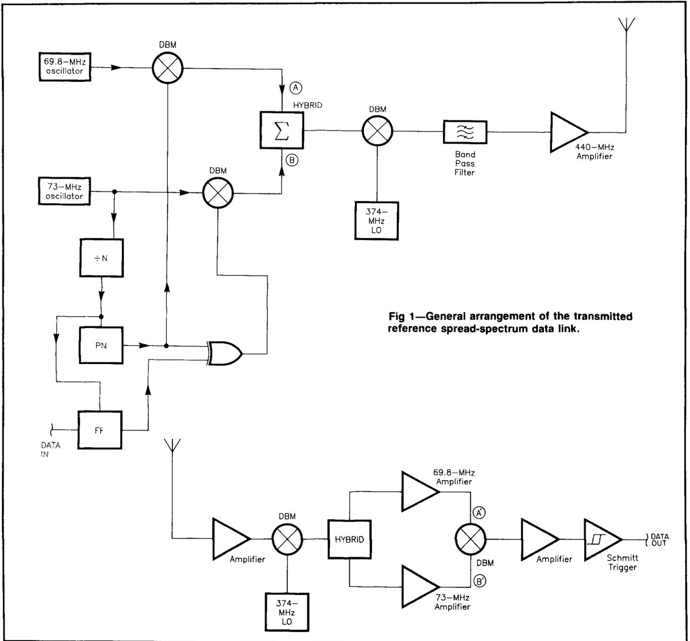
Fig 1—General arrangement of the transmitted reference spread-spectrum data link.
