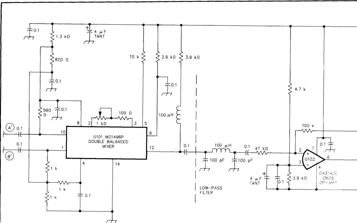
Fig 4—Demodulator circuit.
