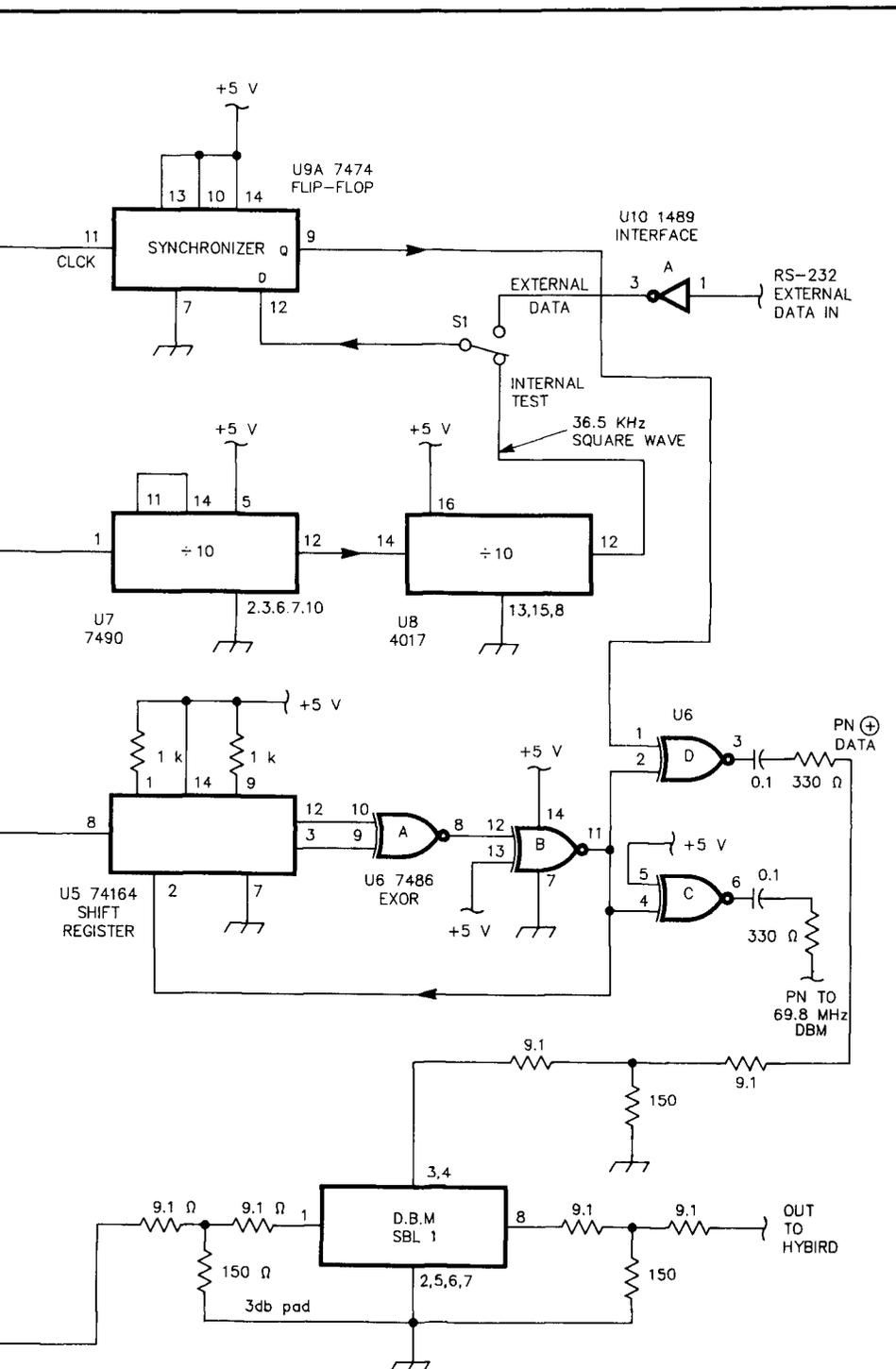
Fig 3—Transmitter circuit.
