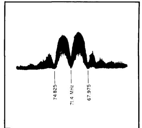
Fig 2—Output of transmitter summing hybrid.
