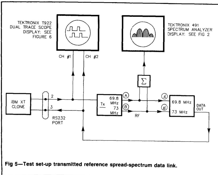
Fig 5—Test set-up transmitted reference spread-spectrum data link.
