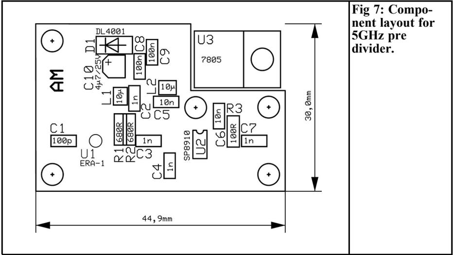
**Fig 7: Component layout for 5GHz pre divider.**
