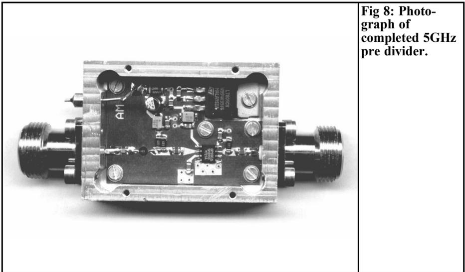
**Fig 8: Photograph of completed 5GHz pre divider.**
