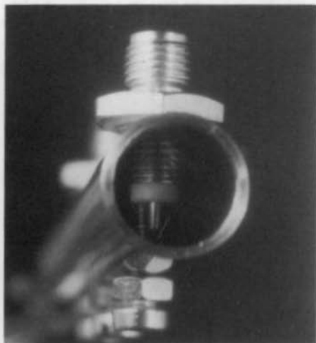
Fig. 3: Coupling by means of the SMA-socket's spigot
