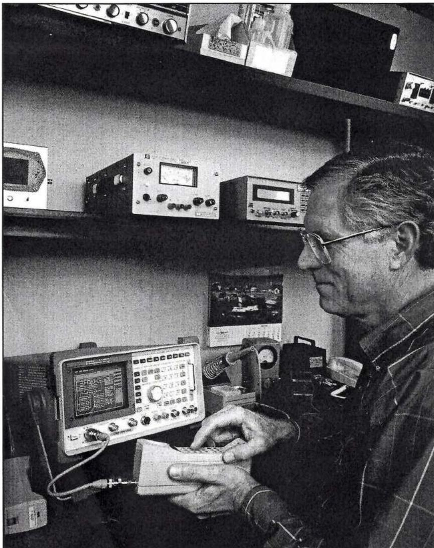
Technician using a test set for cellular analog and digital testing. In addition to hand units, cell sites can be standardized within a cellular system. Photo courtesy of Hewlett-Packard.
