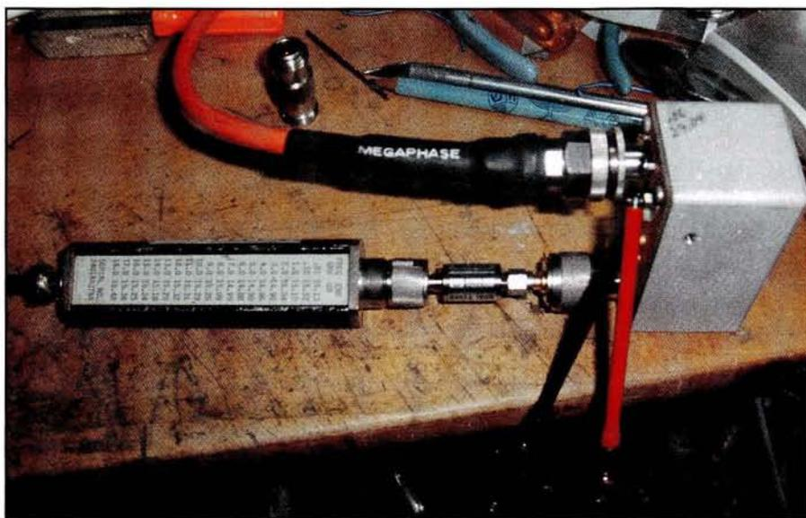
Image 3. Notice the calculated noise source and 10 dB attenuator—a must only for accuracy, but not necessary for tuning and comparing several preamps.
