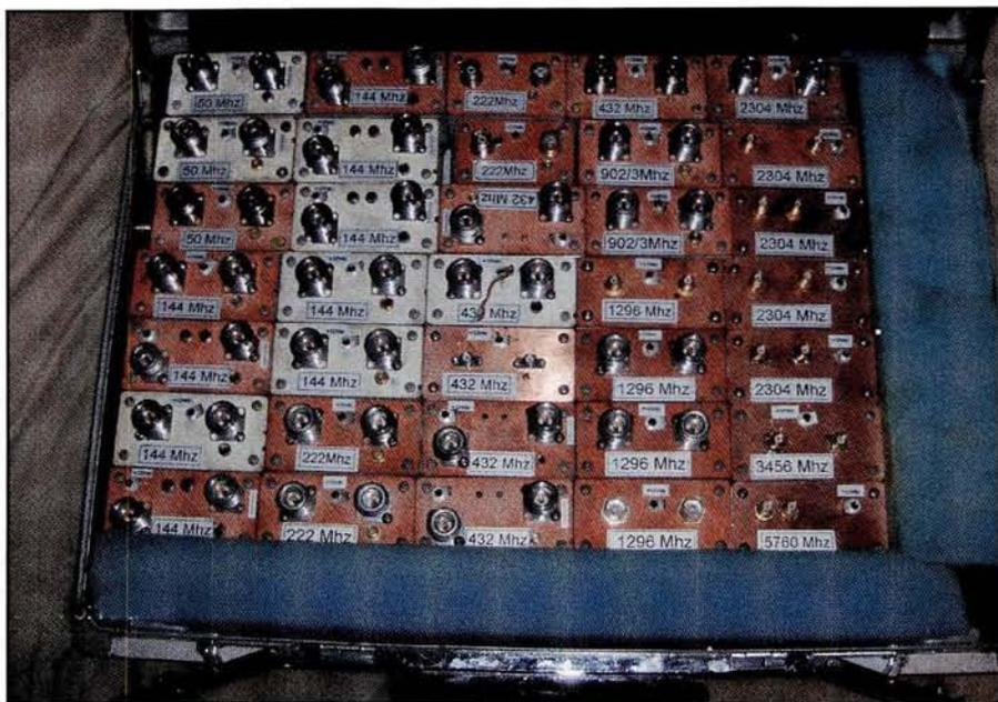
Image 4. My travel case of conference preamps for entry into noise-figure-measuring contests. Notice the many bands and layouts within each band.
