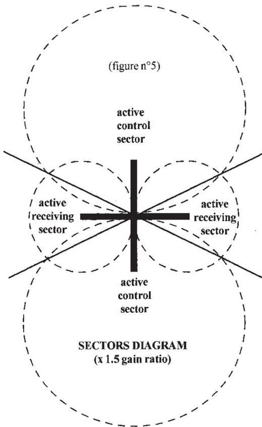
Once again, compare with the single loop antenna (13.4 % of attenuation, or  $-1.25$  dB). The active sector of the main loop has been narrowed definitely by the increase of the control loop gain.
