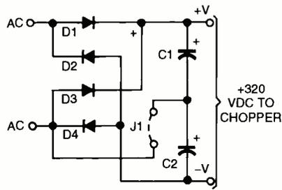
J1 INSTALLED: INPUT = 115V AC
