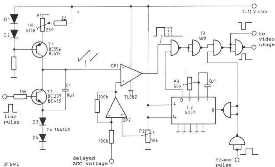
Fig. 1: TV receiver field-strength indicator
