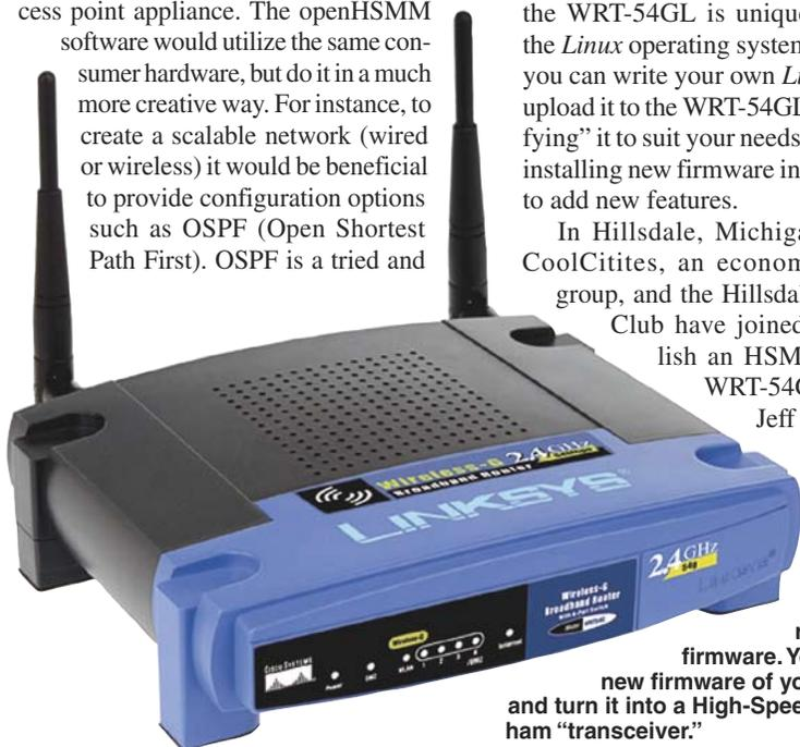
The Linksys WRT-54GL wireless router runs *Linux* firmware. You can upload new firmware of your own design and turn it into a High-Speed Multimedia ham “transceiver.”
