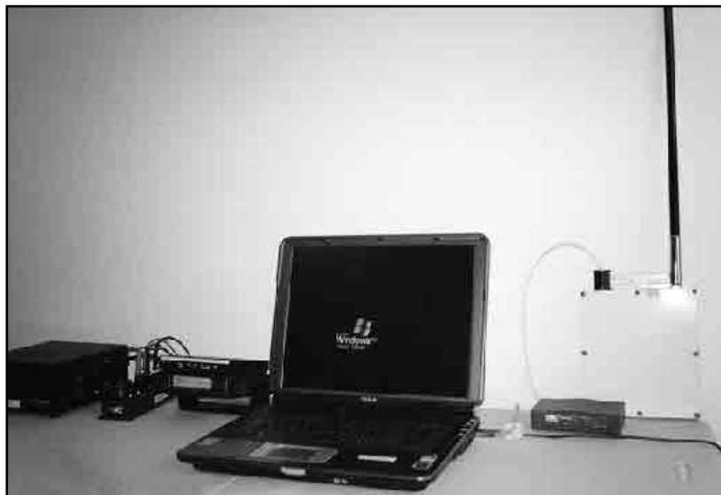
Figure 6 — The components of the integrated network are pictured left to right: Astron power supply, MFJ power strip, Yaesu FT-8800 transceiver with KPC3+ TNC sitting on top, Winbook laptop with Paclink AGW, Paclink Post Office and AGW Packet Engine software installed. To the right of the server is the SMC router and behind the router is the DWL-2100AP modified by NETKROM.
