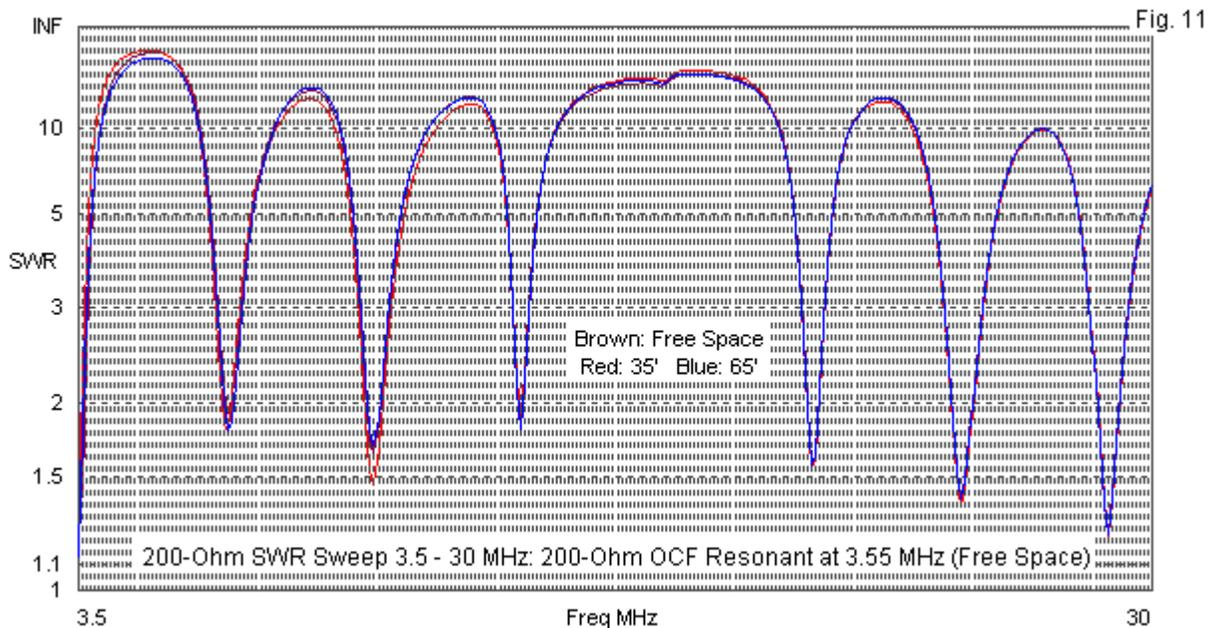
The availability of the 15-meter band within the sweep of the 200-Ω version of the OCF eliminates another band: 17 meters. Moving the feedpoint position closer to the short end of the element results in a coincidence of the new position with the current minimum in this region (about 18 MHz). An azimuth pattern in this region would show a highly aberrant pattern. The SWR curve shows the condition as a dimple in the mid-range high-plateau of SWR values.
