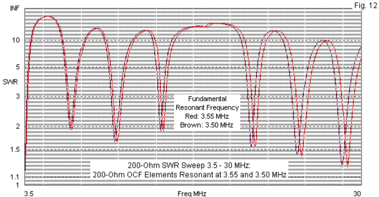
The data in the upper portion of the table, along with the full comparative SWR sweep in **Fig. 12**, show how this simple change moves the harmonic bands downward enough to allow operation in the amateur bands. Only the SWR minimum for 30 meters remains too high in frequency to allow coverage of that amateur allocation (10.1 to 10.150 MHz). However, centering the upper band SWR minimums within the amateur bands to the degree possible does not overcome all limitations of the OCF.
