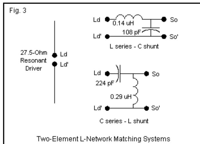
The sketch shows the approximate component values required by each version of the L-network. For each case, we may begin by using lossless components. Although we might assign Qs to the
