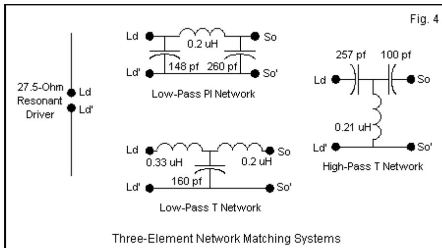
**Fig. 4** outlines the main candidates for matching service. We have low-pass PI and T configurations and a high-pass T arrangement. (A low-pass T is also possible but hardly ever
