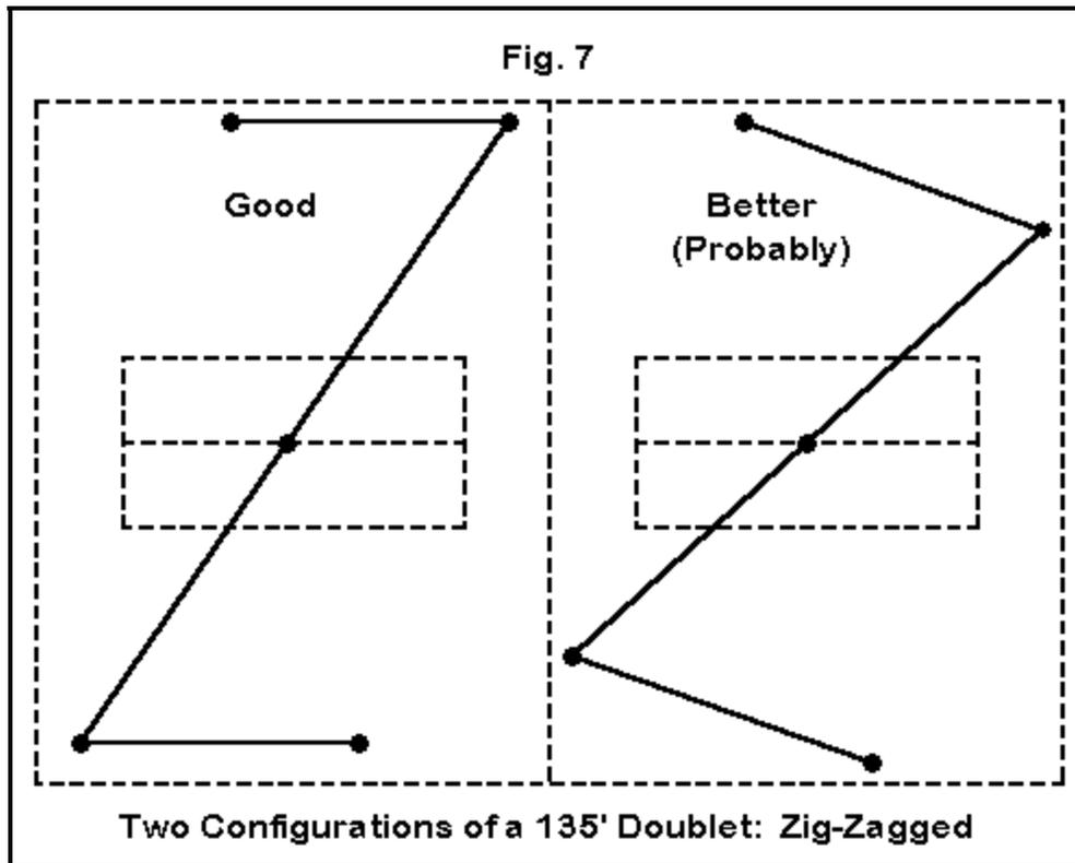
Perhaps the ultimate utility of the zig-zag doublet is to fit a full 80- meter length into a fairly restricted yard size, as suggested in **Fig. 7**. running the antenna diagonally across the yard for the available space and then tilting the wires back along the yard lines (assuming supports are available) can make a multi-band doublet available to almost anyone.
