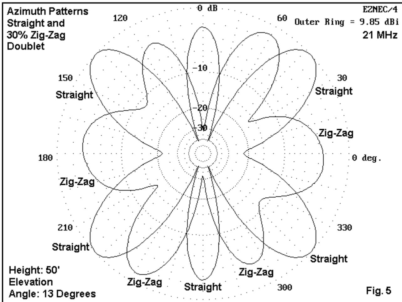
At 21 MHz, the normal and the zig-zag patterns almost oppose each other, with zig-zag lobes filling normal nulls and vice versa. Once more, the normal doublet shows a higher maximum gain (by about 1 dB), but the zig-zag doublet tends to have shallower nulls.
