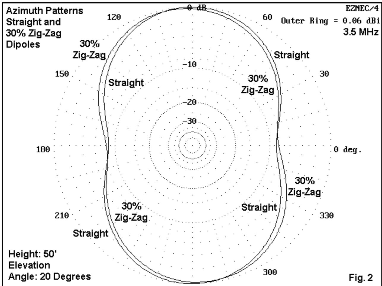
As the zig-zag involves more than 30% of the wire on each side of center, the pattern tilt becomes more extreme, exceeding 10 degrees as the lengths A and B approach each other. We can view this amount of tilt as a disadvantage, or we can put it to use. Suppose the main supports we have will place the broadside pattern some 10 degrees off target for our desired operation. Making the antenna into a zig-zag dipole can put us back on target.
