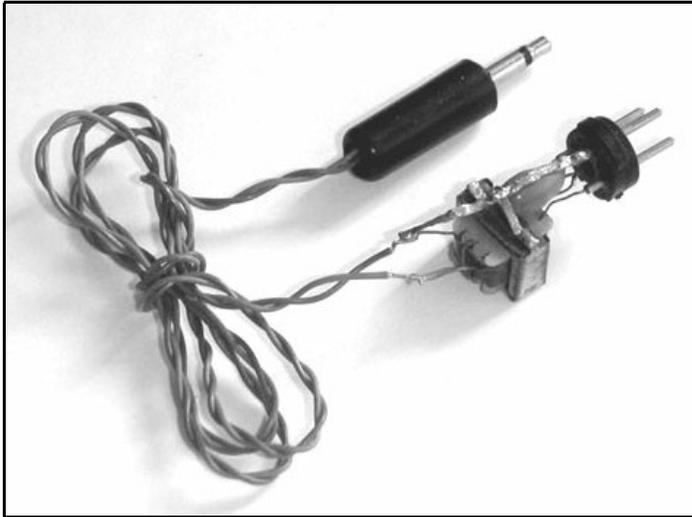
**Fig 6: Audio transformer plug-in for Signal Detector.**
