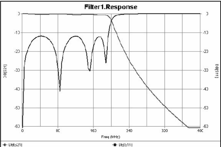
**Fig 9: Response curve of the low pass filter.**
