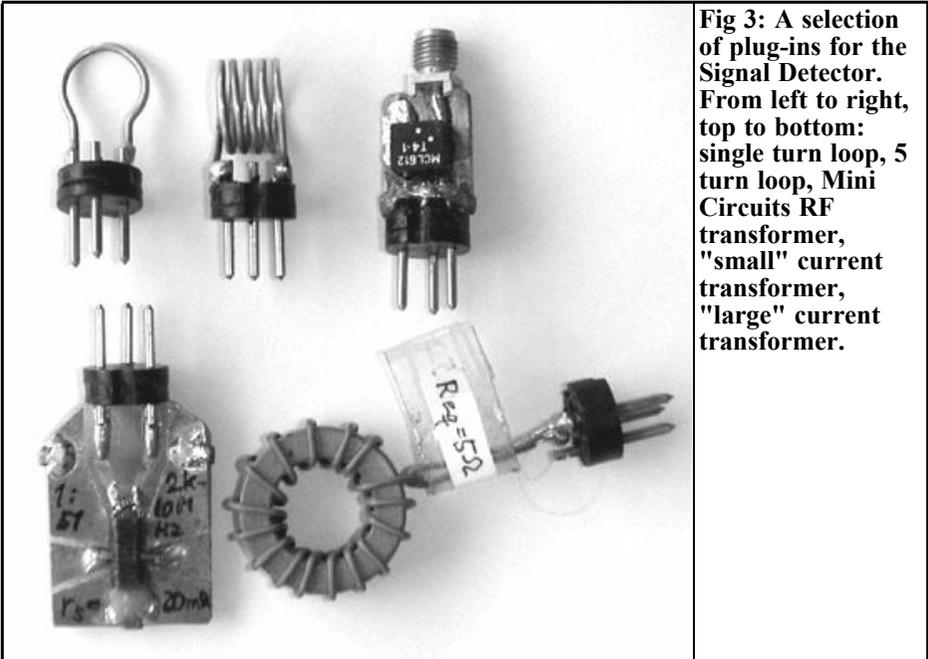
**Fig 3: A selection of plug-ins for the Signal Detector. From left to right, top to bottom: single turn loop, 5 turn loop, Mini Circuits RF transformer, "small" current transformer, "large" current transformer.**
