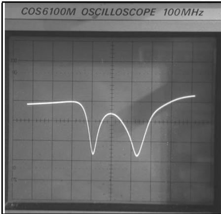
**Fig 10: Return loss of a band pass filter. The span of the display is about 50MHz. It shows that the filter is no good because the return loss rises to zero between the dips, it should dip through the entire band.**
