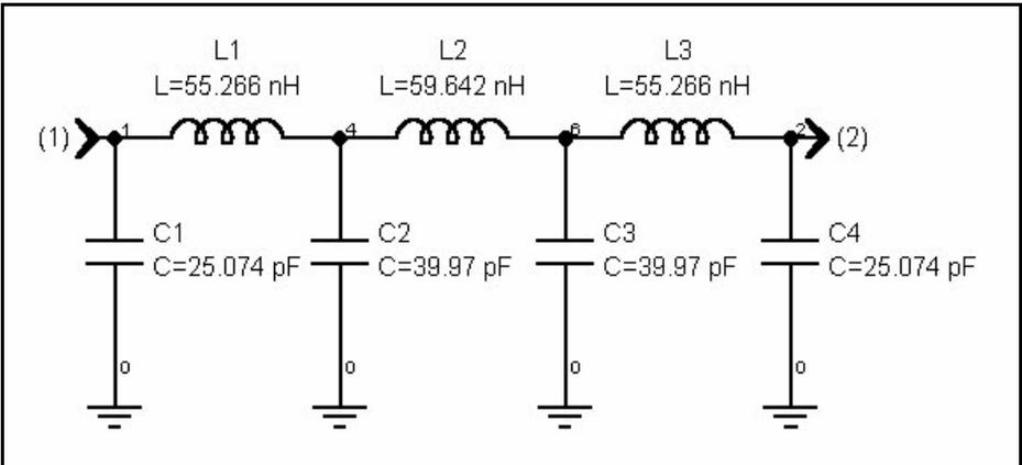
**Fig 8: Circuit diagram of the low pass filter.**
