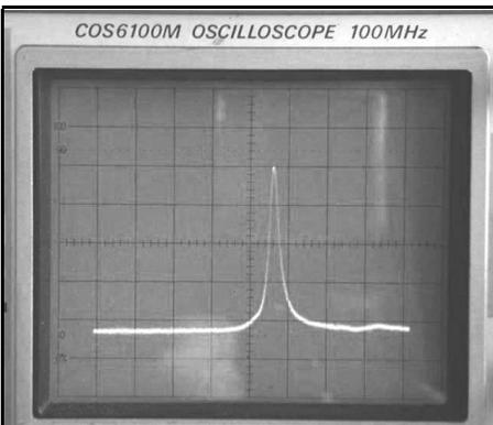
**Fig 5: Output of antenna measurement on an oscilloscope.**
