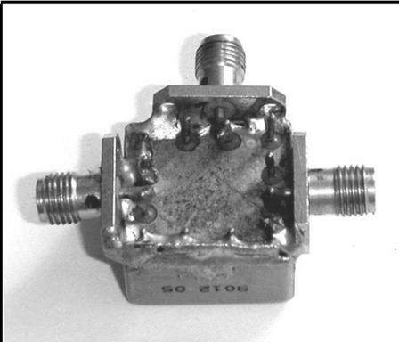
**Fig 12: Mini Circuits reflectometer**
