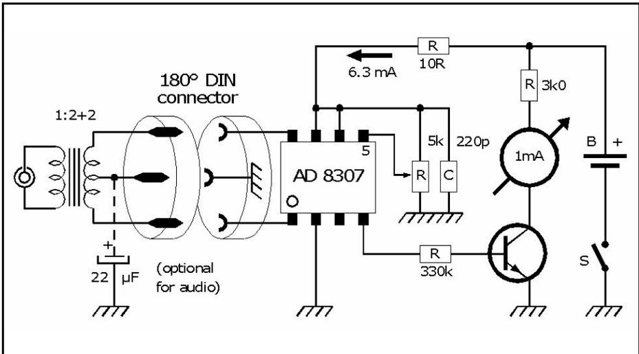
**Fig 2: Circuit diagram of the Signal Detector.**
