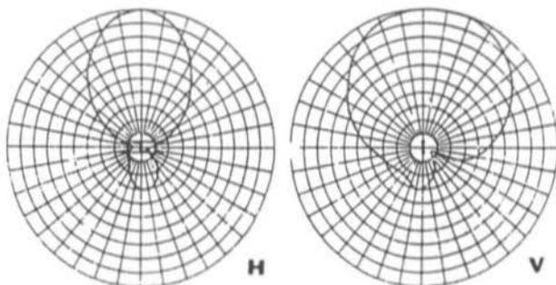
Fig.1 Directional diagrams of the HB9CV antenna
