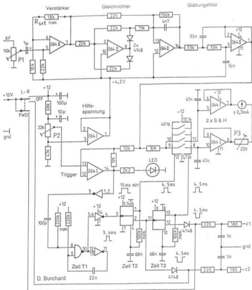
Fig.8 Circuit of the Control and Display electronics
