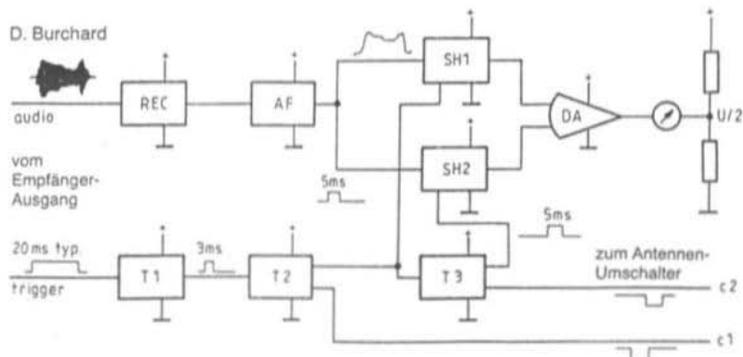
Fig.7 Principle of the Control and Evaluation circuit:
