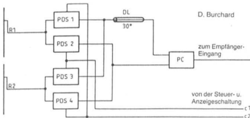
Fig.5 Principle of the Directionality Switch on the Antenna: R = radiator
