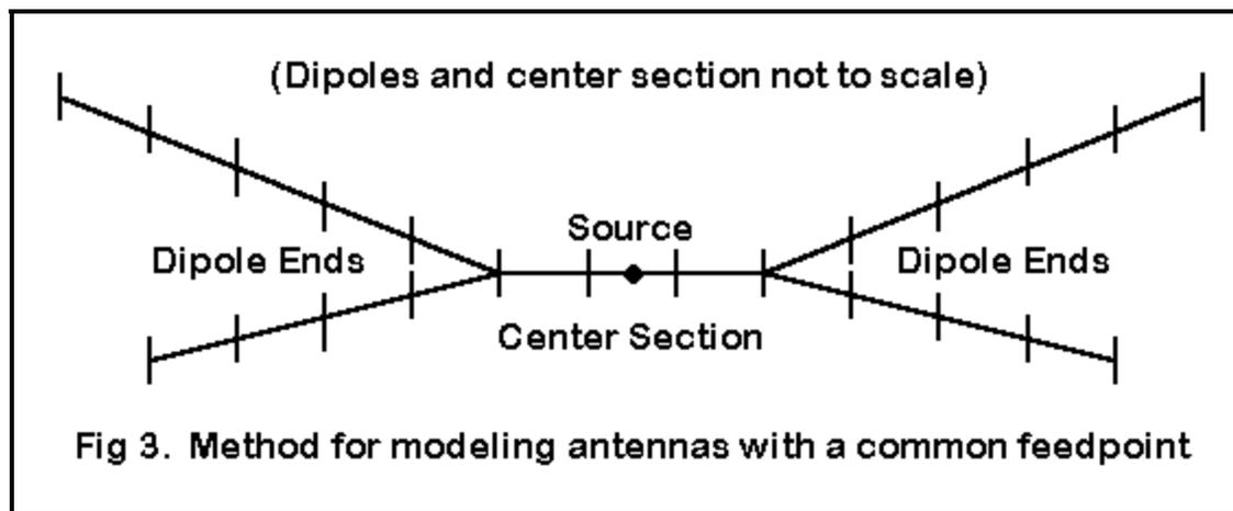
The simple work-around is also shown in Figure 3: adding a small common section of wire for the source and joining the diverging elements to the ends of this wire. Recommendations for this segments include a minimum length of 0.02 wavelength and 3 segments. Equally important, the adjoining segments of the diverging wires should be about the same length as those in the center section.
