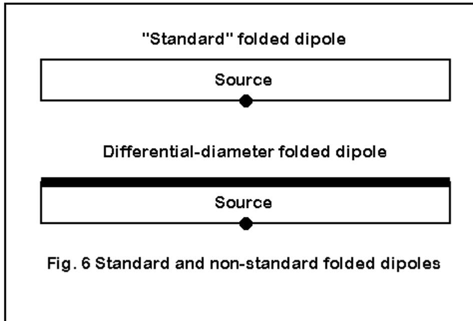
Folded dipoles using dissimilar diameter wires add another dimension to the NEC-2 limitations. Consider two folded dipoles, as shown in Figure 6. One consists of 2 parallel wires 0.5" in diameter spaced 0.25' apart and 16.1' long for 28.5 MHz. The other consists of one 0.5" diameter wire and one #12 (0.808" diameter) wire, also 0.25' apart and 16.2' long for 28.5 MHz. The results of modeling these antennas in both MININEC and NEC-2 are as follows:
