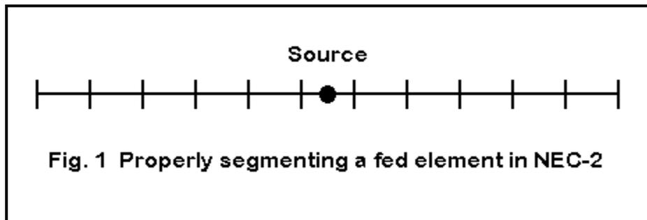
Segment length should be under 0.1 wavelength long, with 0.05 wavelength preferred (about 10-11 segments per half-wavelength). Segments shorter than 0.001 wavelength should also be avoided. For reference, the following table provides a ham band list of the maximum and minimum recommended segments lengths.
