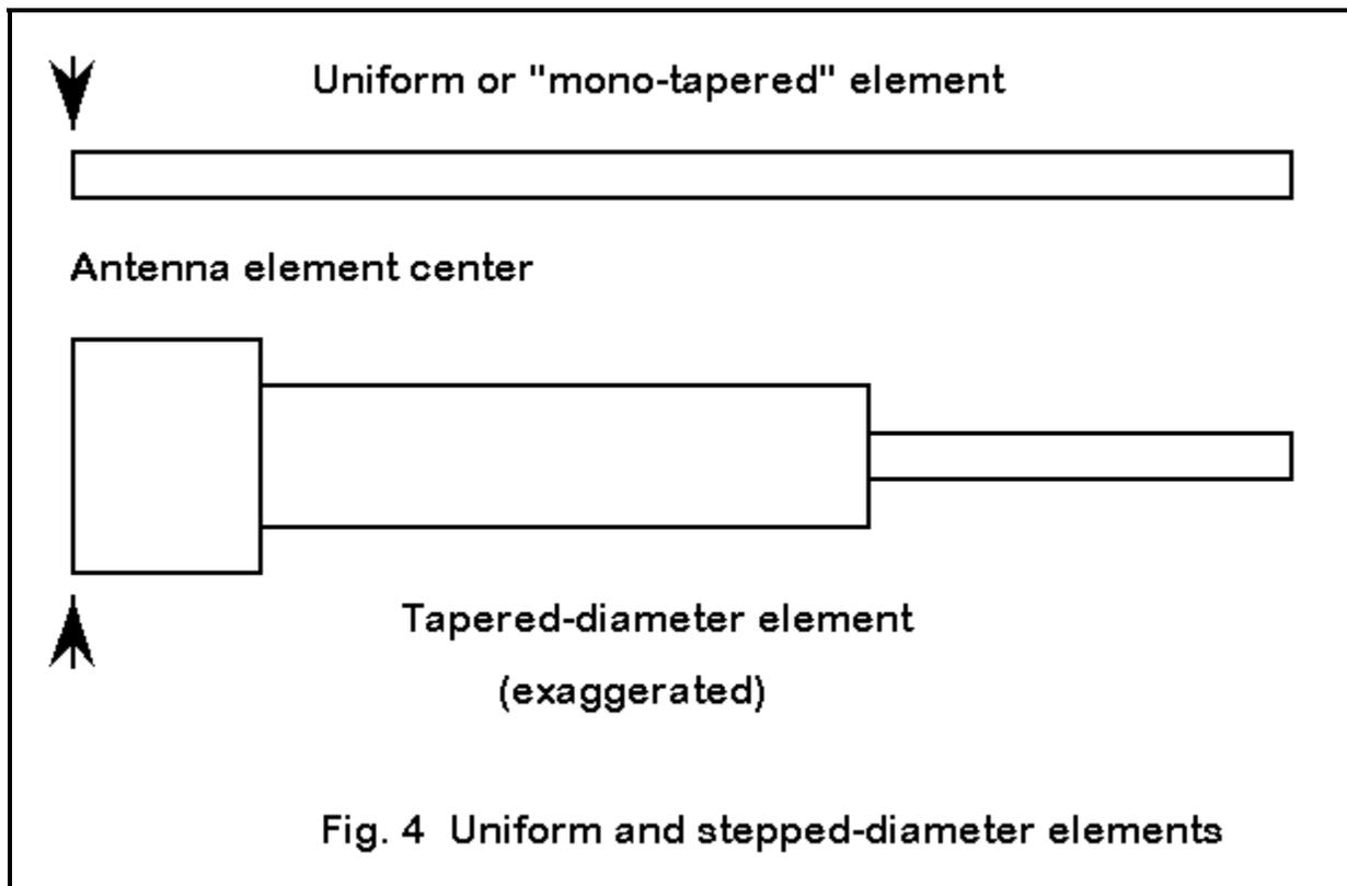
Fig. 4 Uniform and stepped-diameter elements
