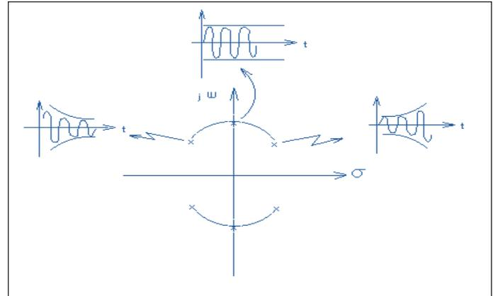
▲ Figure 2. Frequency domain root locus and the corresponding time domain response.
