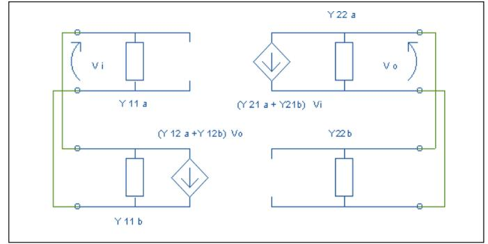
▲ Figure 8. Rearrangement of the Figure 3 oscillator model for open loop gain circulation.
