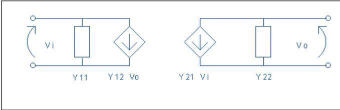
▲ Figure 6. Two port network model of an amplifier.
