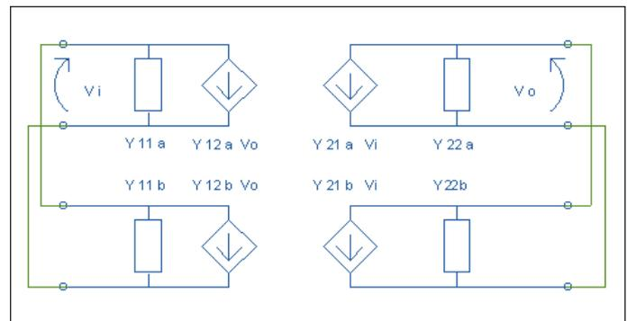
▲ Figure 3. As oscillator circuit modeled as a shunt-shunt connection of two-port networks.
