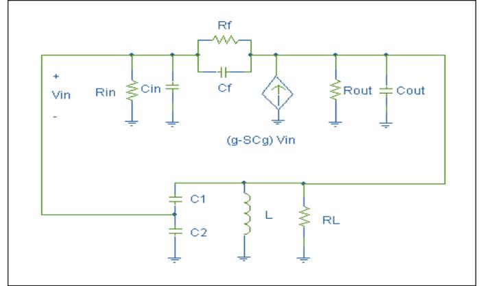
▲ **Figure 10. Variational model of a Colpitts Oscillator with a non ideal amplifier.**
