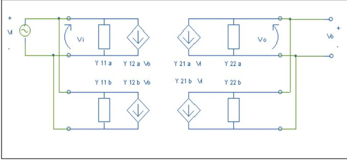
▲ Figure 4. Setup used to evaluate  $A \times H_1(S)$ .
