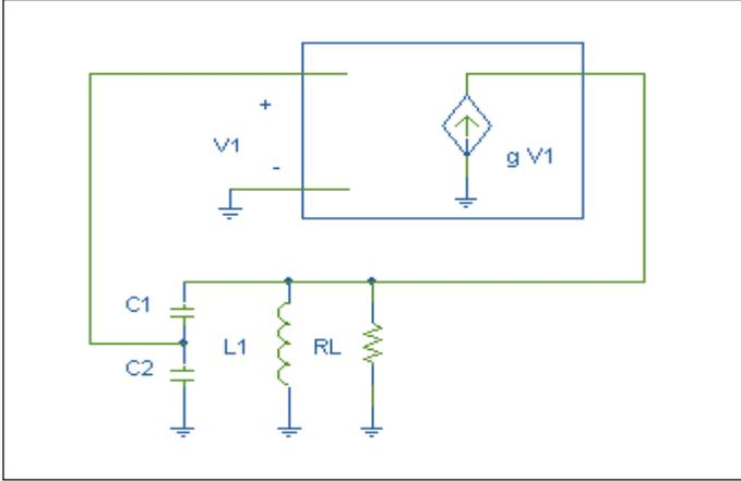
▲ **Figure 9. Colpitts oscillator with an ideal transconductance amplifier.**
