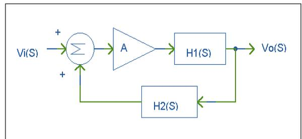
▲ Figure 1. Block diagram of an amplifier with feedback.
