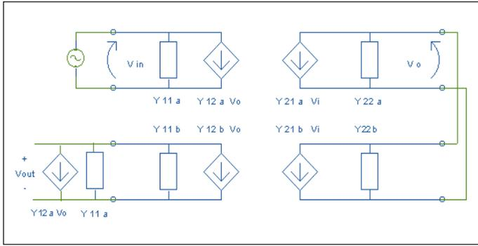
▲ Figure 7. Open loop gain evaluation circuit.
