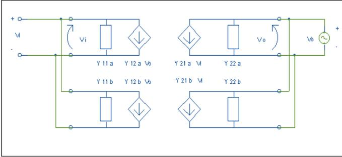
▲ Figure 5. Setup used to evaluate  $H_2(S)$ .
