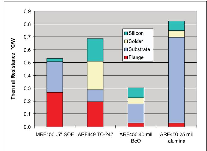
▲ Figure 1. Comparison of thermal stacks.
