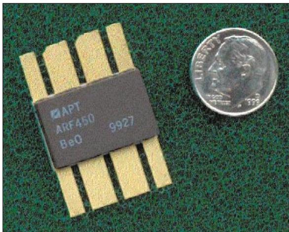
▲ Development of the ARF450 required a complete re-analysis of thermal design.
