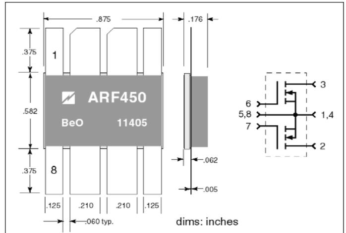
▲ Figure 2. ARF 450 package dimensions and connections.
