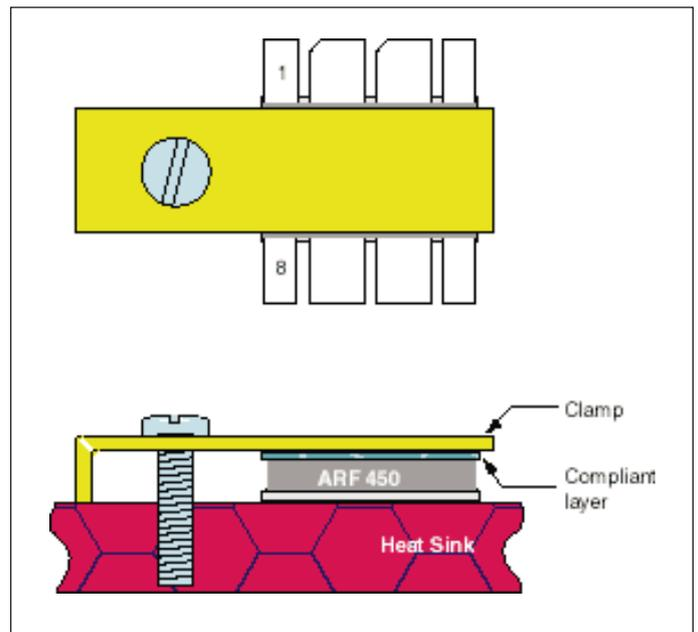
▲ Figure 3. Mounting the ARF450 package.
