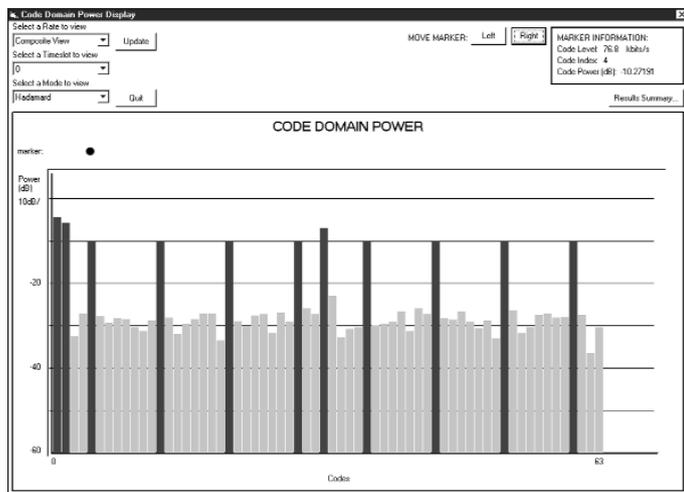
▲ **Figure 6. Code-domain power measurement of cdma2000 SRI signal (instrument has specific cdma2000 capability).**
