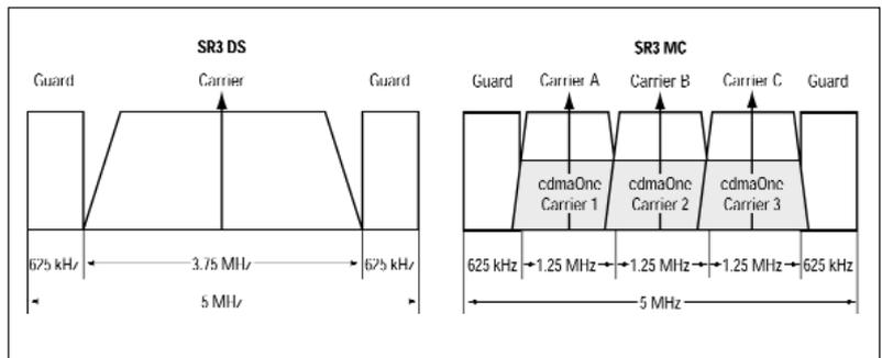
▲ **Figure 2. Bandwidth limits for SR3DS and SR3 MC.**
