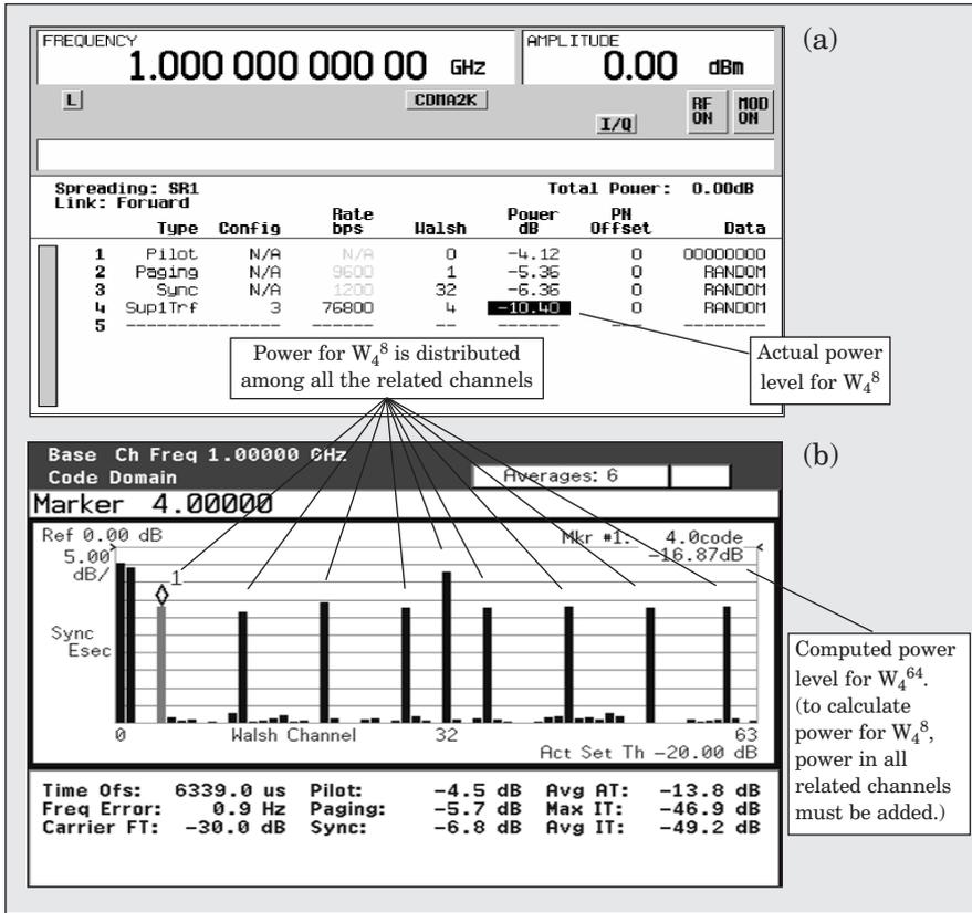
▲ **Figure 5. (a) Signal generation and (b) code-domain power for a cdma2000 signal with pilot, paging and sync channels and an RC3 (76.8 kbps) channel ( $W_4^8$ ). The measurement is performed using an instrument with code-domain power capability for cdmaOne.**
