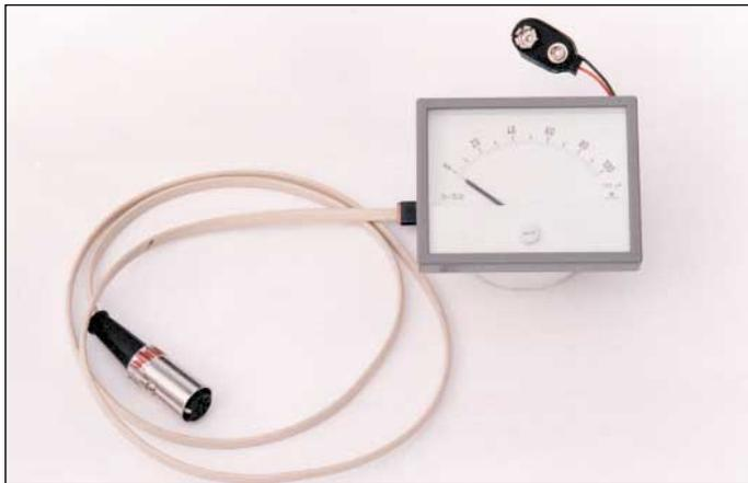
▲ **Figure 13.** LogProbe is permanently hooked up to a meter, and if one needs to look at the response with an oscilloscope, the probe is clipped to the back of the meter.
