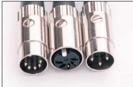
▲ Figure 2. Both a 3-pin and a 5-pin plug fit into LogProbe.
