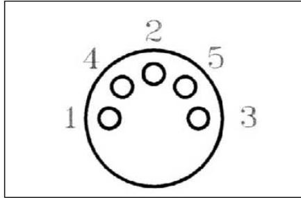
▲ Figure 1. LogProbe front view showing connector pins.
