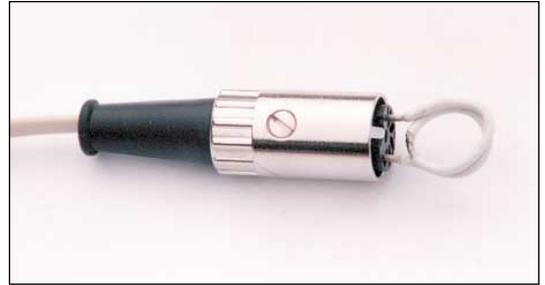
▲ Figure 3. A simple pickup for magnetic fields.
