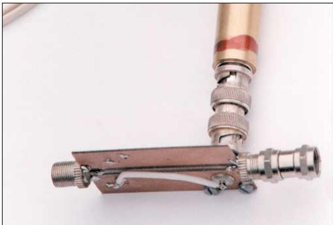
▲ **Figure 16.** LogProbe with a directional coupler.
