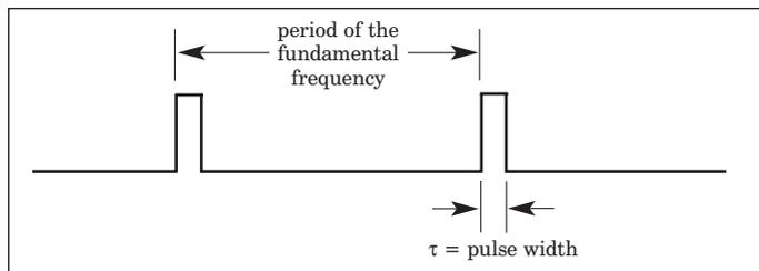
■ Figure 1. Waveform which will create a uniform "comb" over a wide frequency span.
