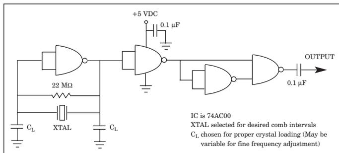
■ Figure 3. Schematic of the simple comb generator.
