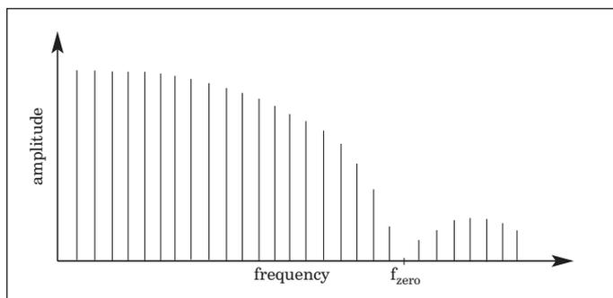
■ Figure 2. The amplitude of the output spectrum has a  $\sin(x)/x$  response with the first zero at  $f_{\text{zero}} = 1/\tau$ .
