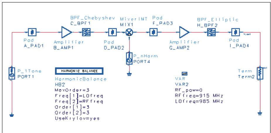
▲ Figure 15. Schematic used for the harmonic balance simulation of the receiver, including a multitone local oscillator source. This simulation used library models for the RF and IF filters.
