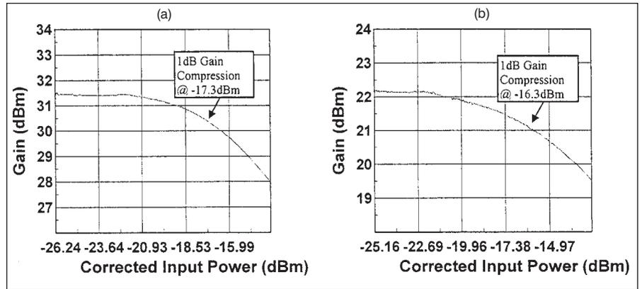
▲ Figure 4. Measurement of input 1 dB gain compression power for the 915 MHz RF amplifier (a) and 70 MHz IF amplifier (b).
