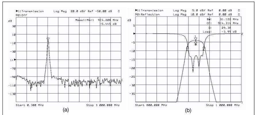
▲ Figure 6. Measured response of the 915 MHz pre-select filter. The broadband response (a) shows out-of-band performance. Narrowband passband and return loss measurements are in (b).
