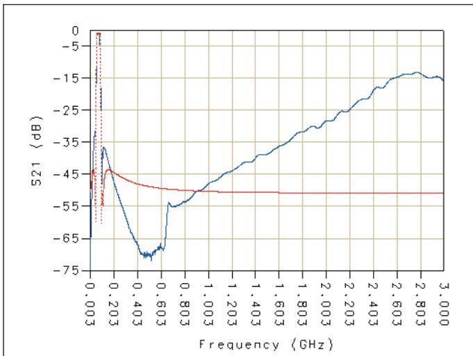
▲ **Figure 18.** Comparison between  $s_{21}$  for the library model of the IF filter and the measured frequency response of the filter used in the receiver.
