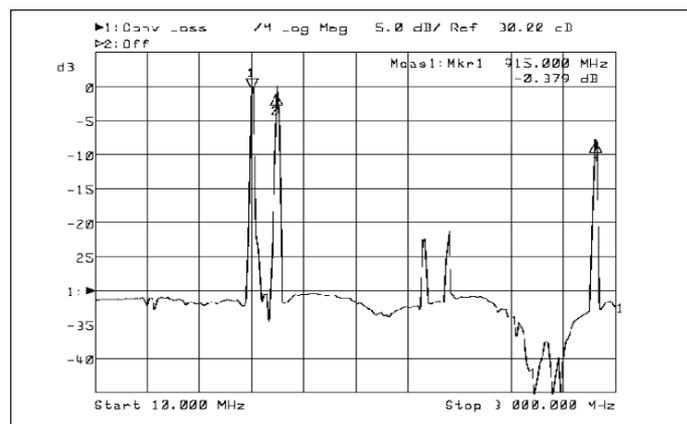
▲ Figure 12. Measured small-signal sweep results with the RF pre-select filter removed.
