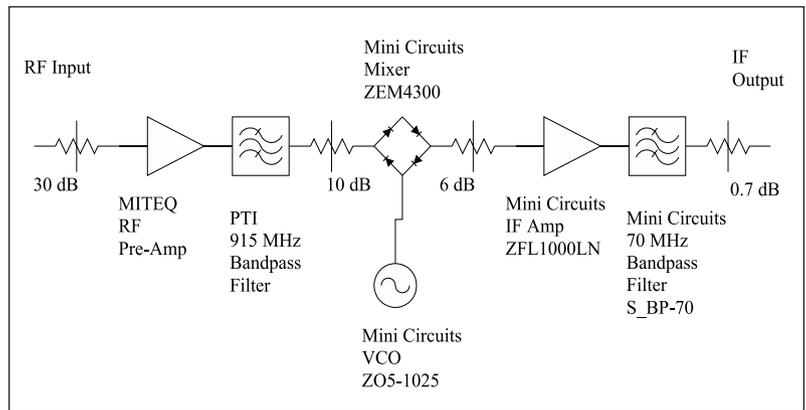
▲ Figure 1. Block diagram of the 915 MHz receiver subsystem.
