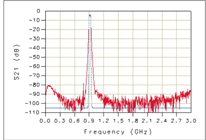
▲ **Figure 17.** Comparison between  $s_{21}$  for the library model of the RF filter and the measured frequency response of the filter used in the receiver.
