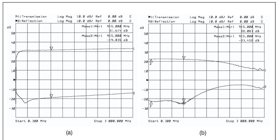
▲ Figure 3. Broadband (0-3000 MHz) measured transmission and reflection responses for the MITEQ (a) and Mini-Circuits (b) amplifiers. The markers are at 70 MHz and 915 MHz. The input signal level was about  $-30$  dBm.
