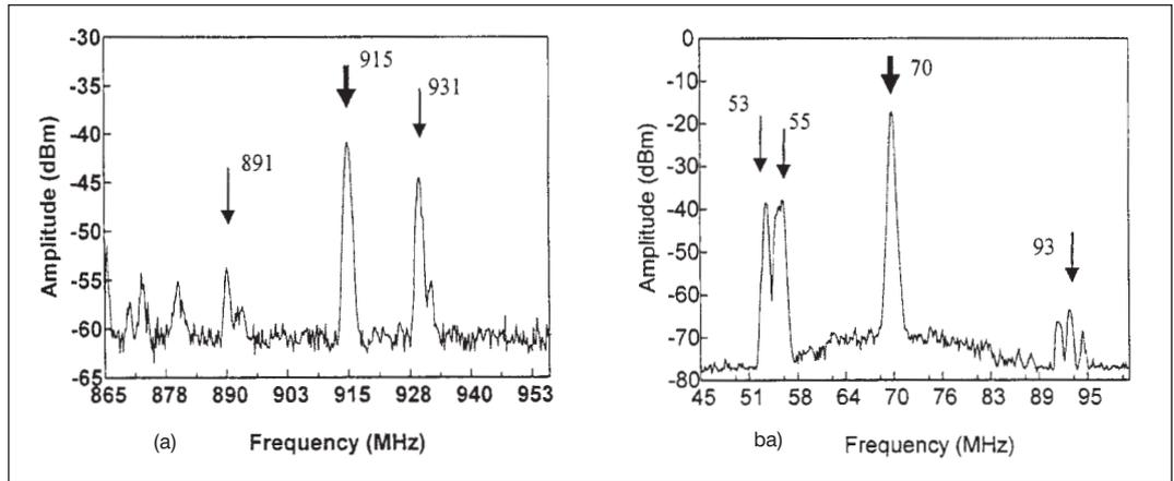
▲ **Figure 19. RF input (a) and IF output (b) spectrum analyzer displays of the frequency and amplitude of the received spectrum, using an antenna to receive a 915 MHz test signal along with ambient signals. For (a), the receiving antenna is connected directly to the SA, while (b) was measured with the antenna connected to the subsystem input and the IF output connected to the SA.**
