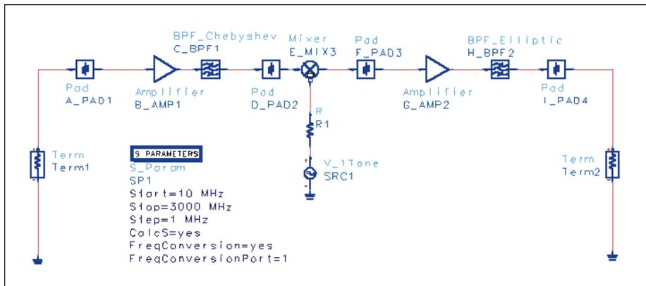
▲ Figure 9. Schematic used for the small signal sweep of the subsystem.
