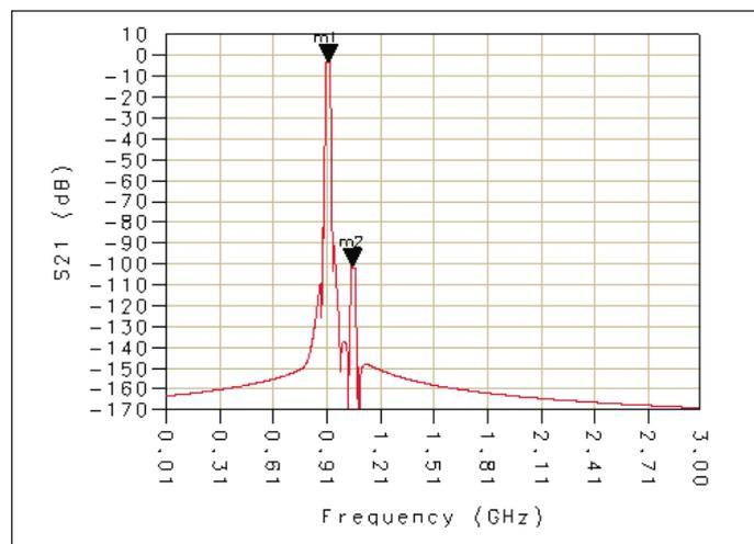
▲ Figure 10. Simulated small-signal sweep results including the RF pre-select filter.
