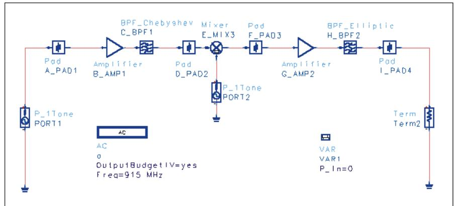
▲ **Figure 8. Schematic used for the power budget analysis.**
