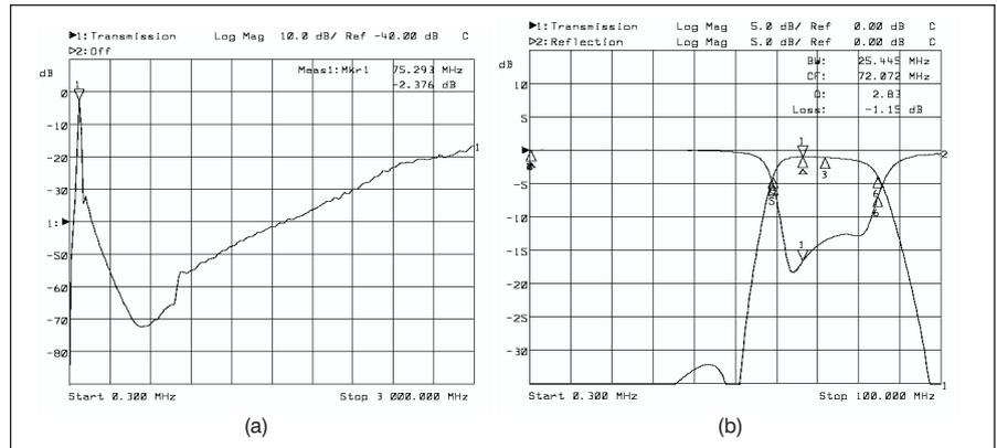
▲ **Figure 7. Broadband (a) and narrowband (b) responses for the Mini-Circuits 70 MHz IF bandpass filter. The broadband response shows that out-of-band rejection degrades at high frequencies.**
