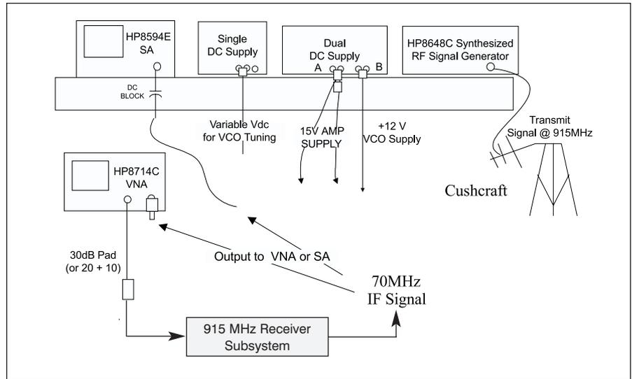
▲ Figure 2. The basic test bench used for characterization of the 915 MHz receiver and its components.
