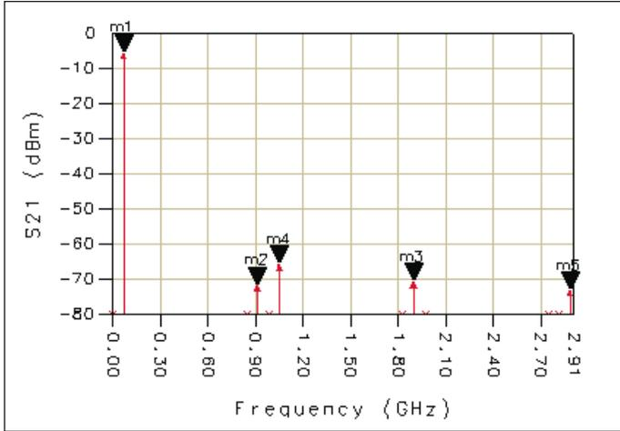
▲ **Figure 16.** Simulation results for the harmonic balance analysis. The markers correspond to the following output products:  $m1 = \text{IF}$ ,  $m2 = \text{RF}$ ,  $m3 = 2 \times \text{LO}$ ,  $m4 = \text{LO}$ ,  $m5 = 2 \times \text{LO} + \text{RF}$ .
