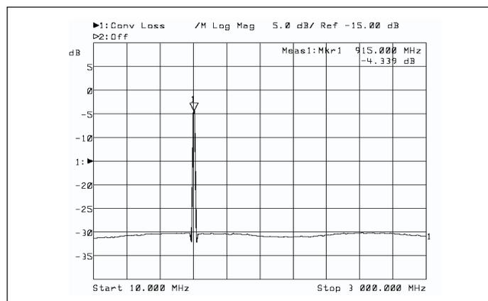
▲ Figure 11. Measured small-signal sweep results including the RF pre-select filter.
