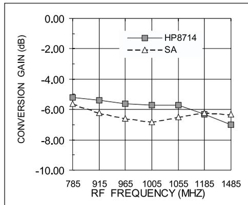
▲ Figure 5. Mixer conversion loss measured with a VNA and SA. The LO is 985 MHz at  $+4$  dBm; RF is  $-20$  dBm.
