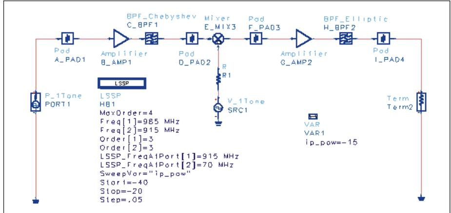
▲ Figure 13. Schematic used for the large-signal sweep of the subsystem.
