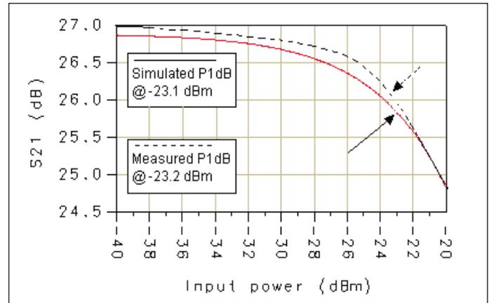
▲ Figure 14. Simulated and measured large-signal sweep results. Note the close agreement.
